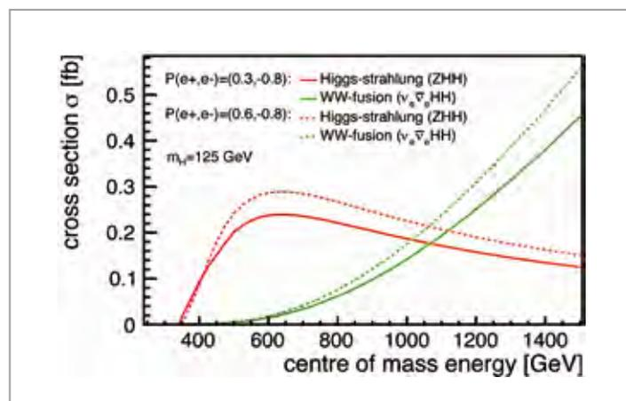
Figure 1 SM cross section for double Higgs production in polarised electron–positron collisions as a function of the centre-of-mass energy [1]. The full lines correspond to the ILC baseline design, which provides a positron polarisation of 30%. The dashed lines correspond to an upgrade to 60% positron polarisation.
