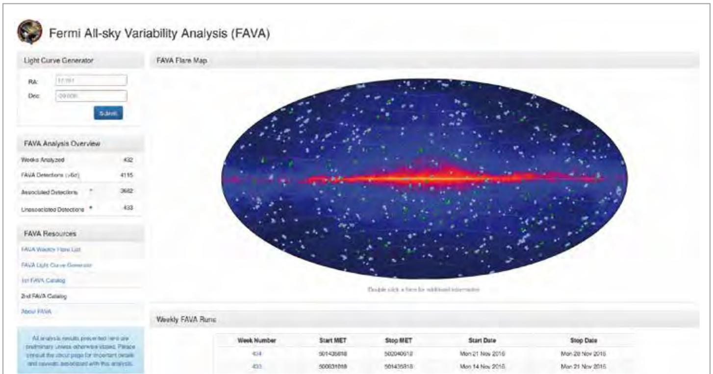
Figure 2: FAVA web page (<http://fermi.gsfc.nasa.gov/ssc/data/access/lat/FAVA/>). Flares are shown as grey and green dots. Photometric light curves can be generated for every position on the sky (upper left panel).
