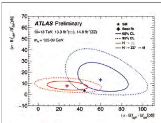
Figure 1 Measurement of the gluon–gluon fusion and vector boson fusion production cross sections in Higgs boson decays to two photons and to four leptons
