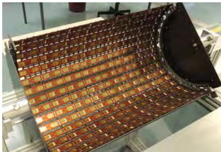
Fourth barrel layer of the CMS pixel detector with half of the mounted modules
