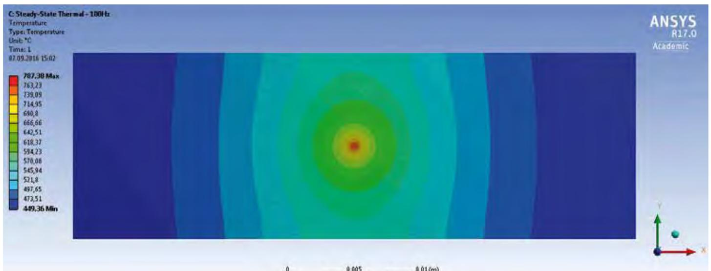
Figure 1 Simulation of the temperature distribution during irradiation; the cyclic load stress is about 250 MPa.
