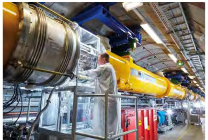
Superconducting accelerator modules (yellow) in the European XFEL tunnel
