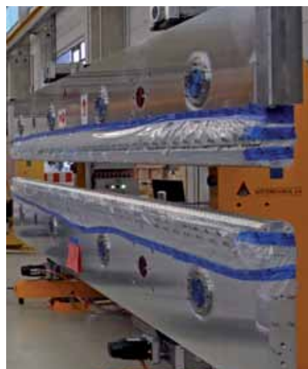
Figure 1 First undulator segments from industrial production: Each five-metre-long segment contains two rows with 207 magnets and has a total mass of eight tons
