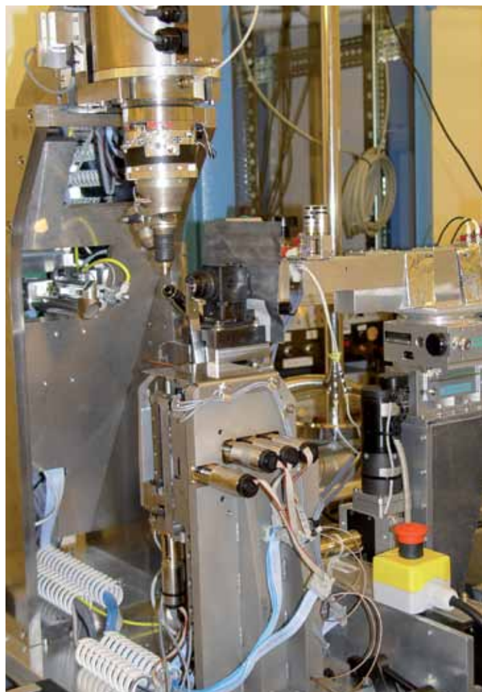
Figure 3 Prototype of a high precision diffractometer with a mini-kappa goniostat mounted on a vertical rotation axis. Development in collaboration with EMBL Grenoble and MAATEL (Voreppe, France).
