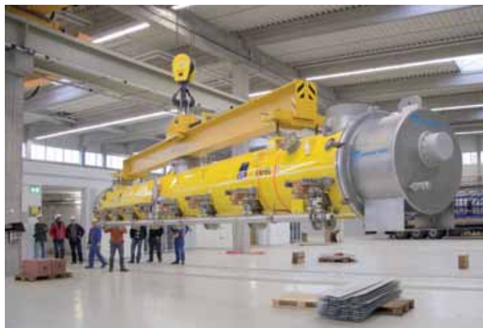
The first accelerator module for the European XFEL is unloaded with the AMTF hall crane.
