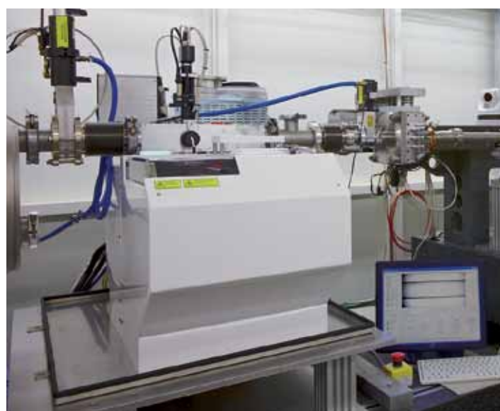
Figure 2 BioSAXS sample changer on beamline P12, developed in collaboration with EMBL Grenoble and the ESRF.
