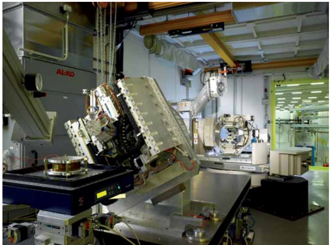
Figure 3 Experimental hutch of the high resolution X-ray diffraction beamline P08 at Petra III
