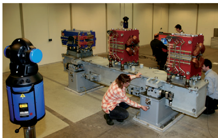
Adjustment of a girder per laser (at left)
