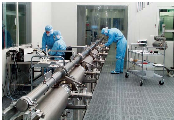
Assembly of the cavities for Module 6 in the cleanroom.
