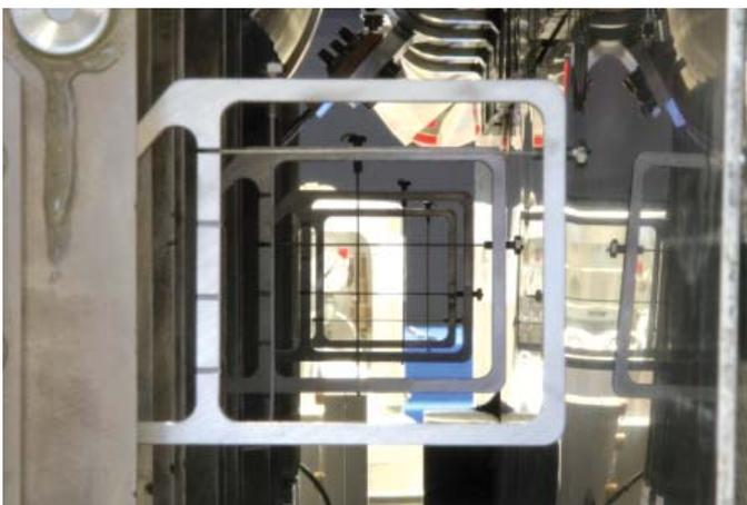
The wire crosses are used to measure the displacement of cavities within the module. The transport did not cause any harm.
