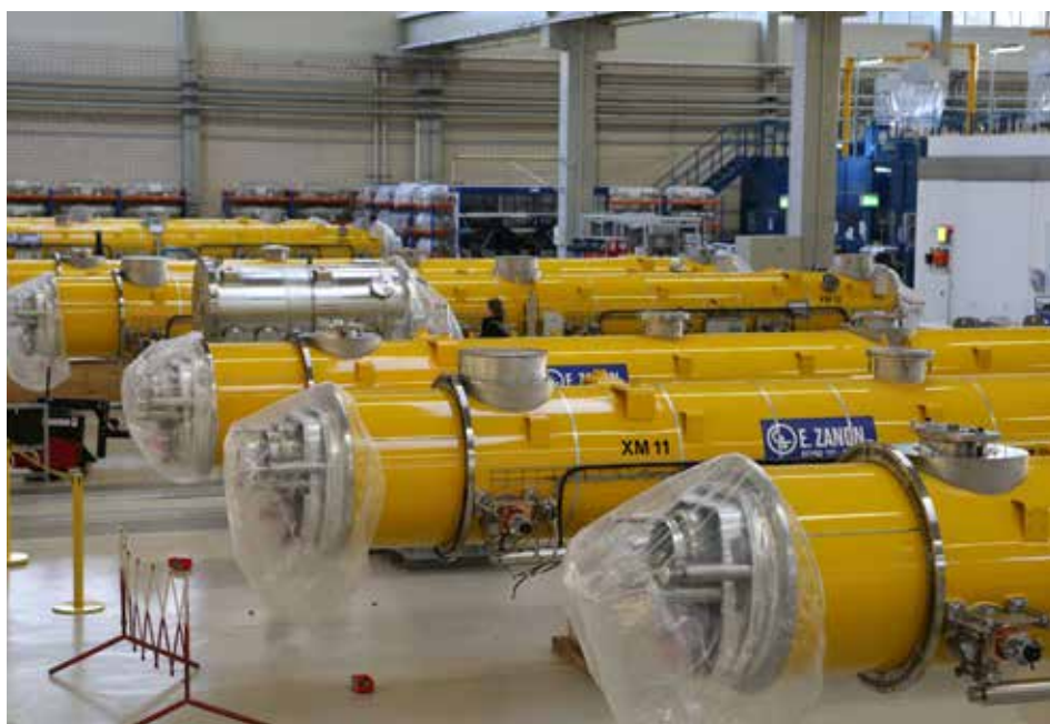
The accelerator modules for the European XFEL will be tested in continuous operation. (Photo: Dirk Nölle)
