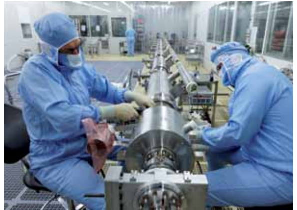
Eight cavities in their helium tank and all other necessary equipment are assembled into a cavity string. This requires extreme precision and extreme cleanliness.
