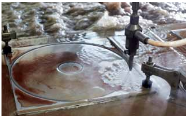
A water jet cutter turns the niobium sheet into the template for the cavity dumbbells.
