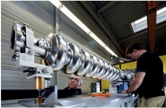
A robot with a specially designed and programmed camera checks whether the welding seams may have the potential of causing a quench and what the inner surface of the cavity looks like.
