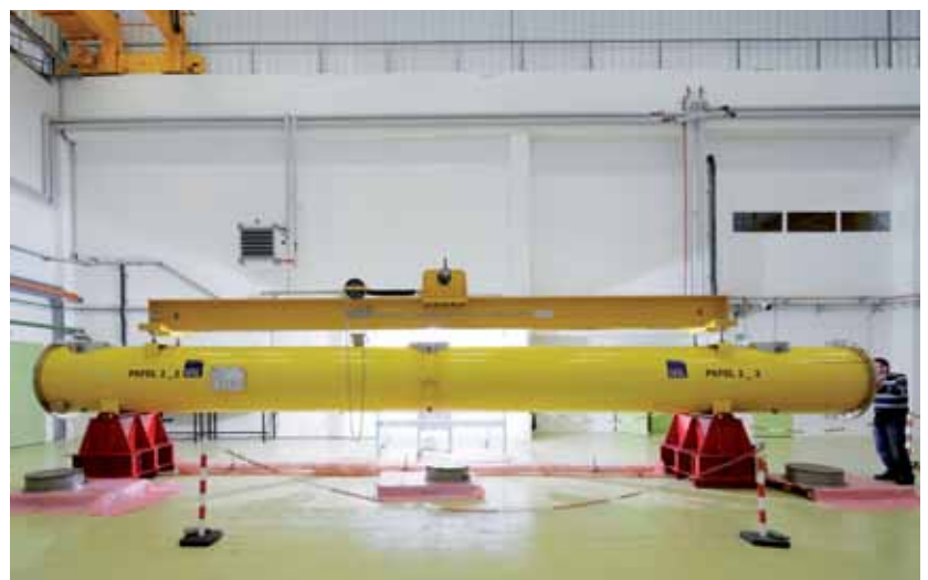
The cavity's final home: the cryomodule. Eight cavities sit in one module, and depending on the accelerator there may be some hundred or more than a thousand of these cryomodules connected to each other in a row.
