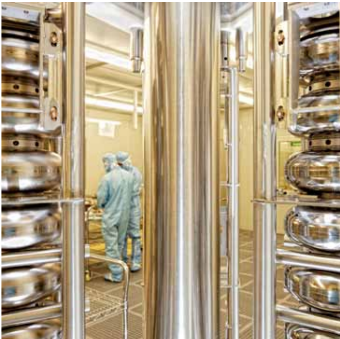
The tried and tested nine-cell cavities are standing ready for assembly.
