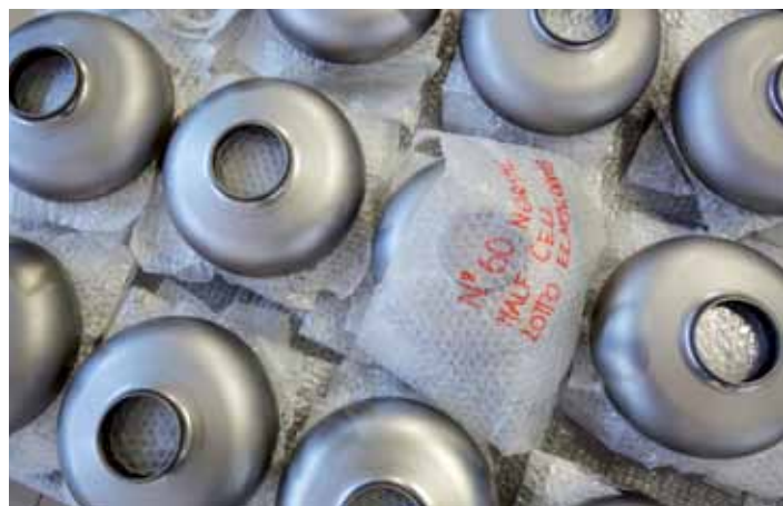
Freshly pressed into form the half cells are ready for welding.
