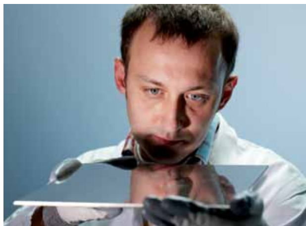
The surface of the niobium sheets is inspected by eye at DESY.
