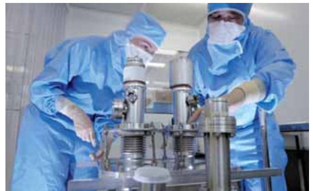
These couplers, built at the French laboratory LAL in Orsay, feed the high frequency into the cavities.
