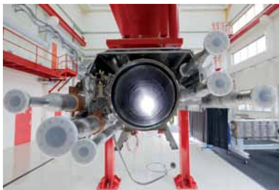
The gaseous helium is returned through this pipe. The cavity string is later attached to this construction before it is inserted into the cryomodule. Here: CEA, Saclay, France.
