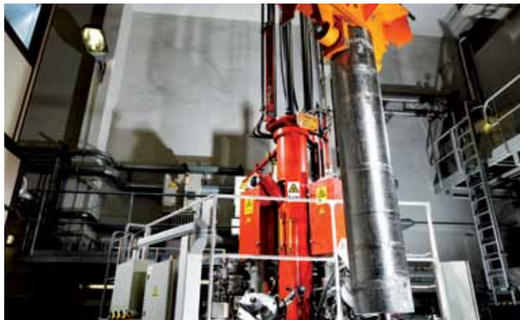
A niobium ingot is lowered into the electron beam melting oven at the German company Heraeus. The melting process turns the already pure niobium into the highly purified material needed for cavity production.
