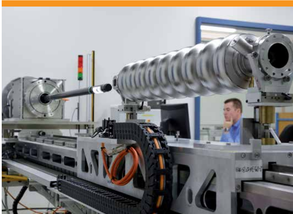
The inspection robot OBACHT examines the superconducting accelerator components from the inside.
