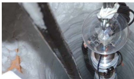
Deployment of a SPATS string in an IceCube drilling hole at the South Pole.
