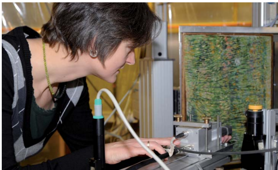
Karen Rickers-Appel at the experiment: With intense synchrotron radiation the team of experts was able to measure very small amounts of mercury and antimony in the lower layers of paint.
