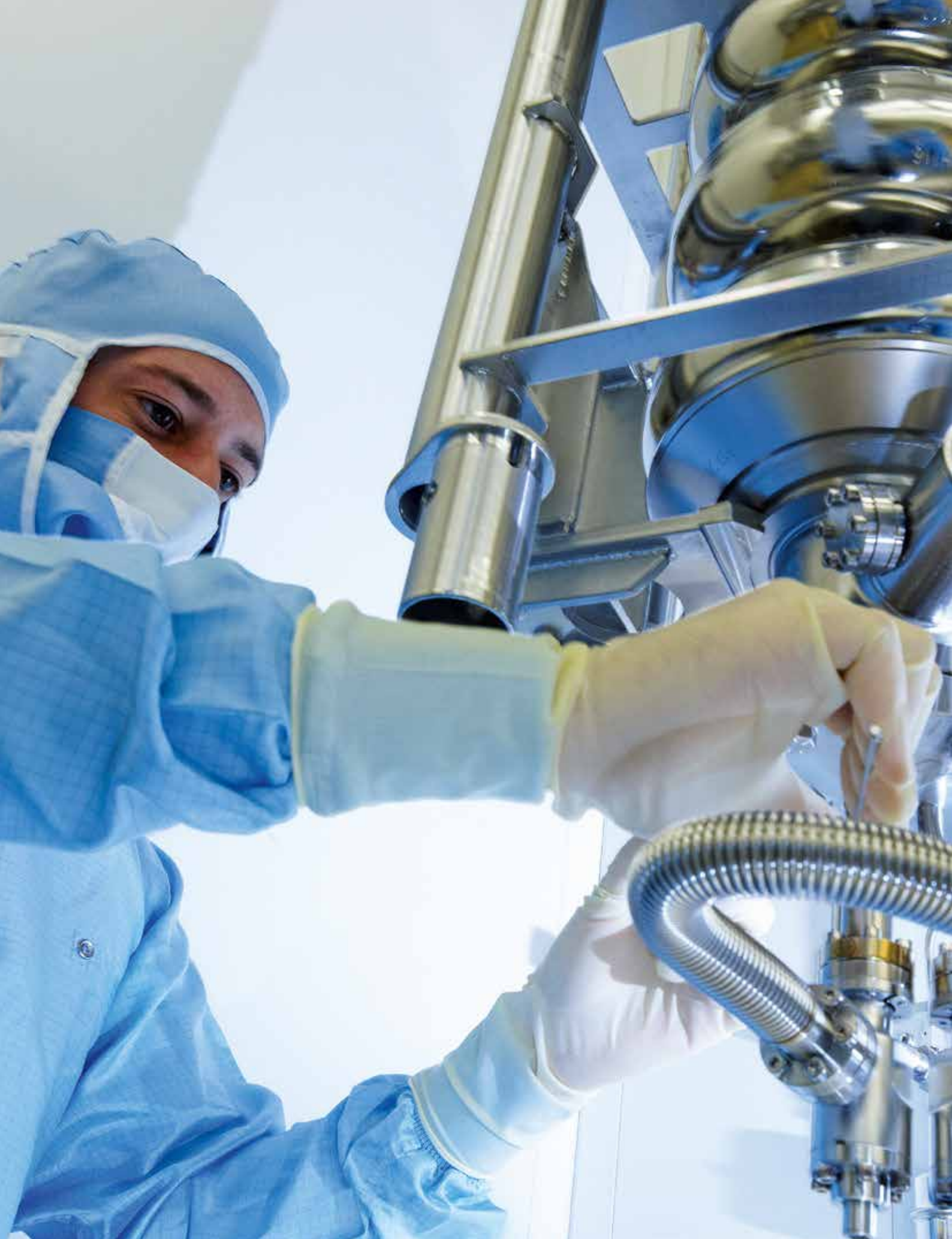
Processing a cavity in the clean room
