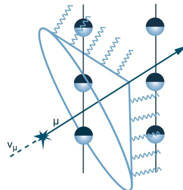
Muon detection through Cherenkov light
