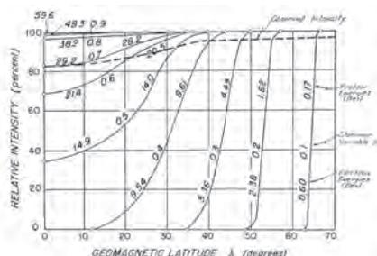
The relative cosmic particle intensity as a function of geomagnetic latitude for minimum energies of electrons and protons
