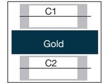
Absorber experiment with Geiger-Müller counters C1 and C2 in coincidence
