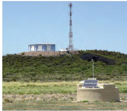
One of the air fluorescence light detector stations on the hill and a water Cherenkov tank on the right
