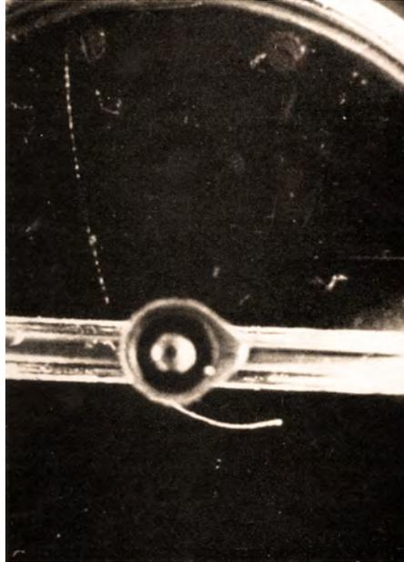
Stereographic photograph of a cloud chamber exposure. A muon enters the chamber from above and comes to rest below.
