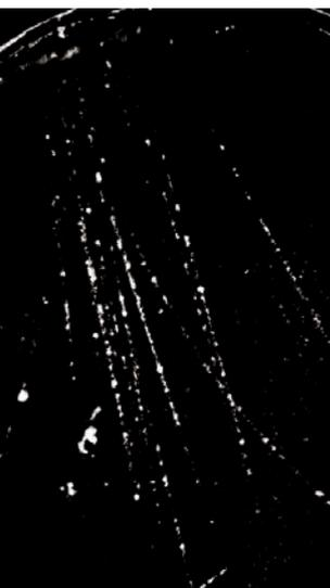
Cloud chamber photograph of a particle shower with about 16 tracks. The divergence of the tracks points to an interaction in the magnet coil.
