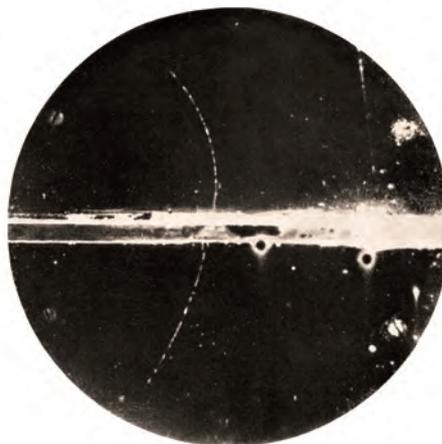
A positron with an energy of 63MeV entering the lead plate from below and leaving the plate with an energy of 23MeV. For a proton, the track length would be ten times shorter.
