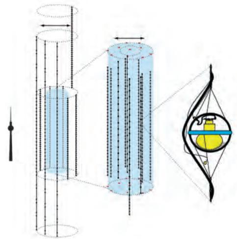
Schematic view of the 19-string AMANDA detector mostly installed at a depth of 1400m–2000m
