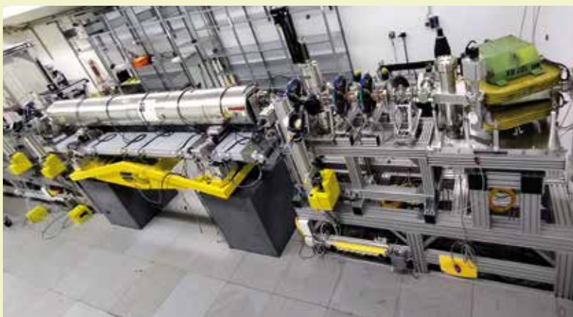
View inside the PITZ extension with the terahertz laser. The undulator that generates the laser radiation is mounted on the yellow frame, the electron beam enters the beamline from the right.
