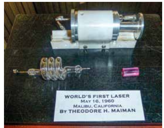
The components of the first ruby laser by Theodore Maiman
