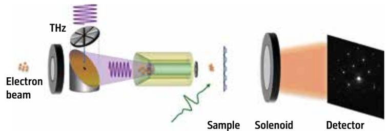
**A** compact electron camera enables researchers to capture the ultrafast internal dynamics of matter. The system fires short bunches of electrons at a sample to take snapshots of its inner structure. It is the first such electron diffractometer that uses terahertz radiation to compress the electron bunches. The short wavelength of the terahertz radiation enables a compact design.
