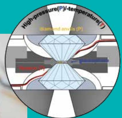
View into a diamond anvil cell (left). To study the water-bearing minerals, the samples can be heated by laser (top).
