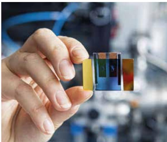
Green electricity for hydrogen production: The organic solar cell layer, which is only 200 nanometres (millionths of a millimetre) thin, converts light with an efficiency of almost 30 percent into electricity, which can be used directly to split water.
