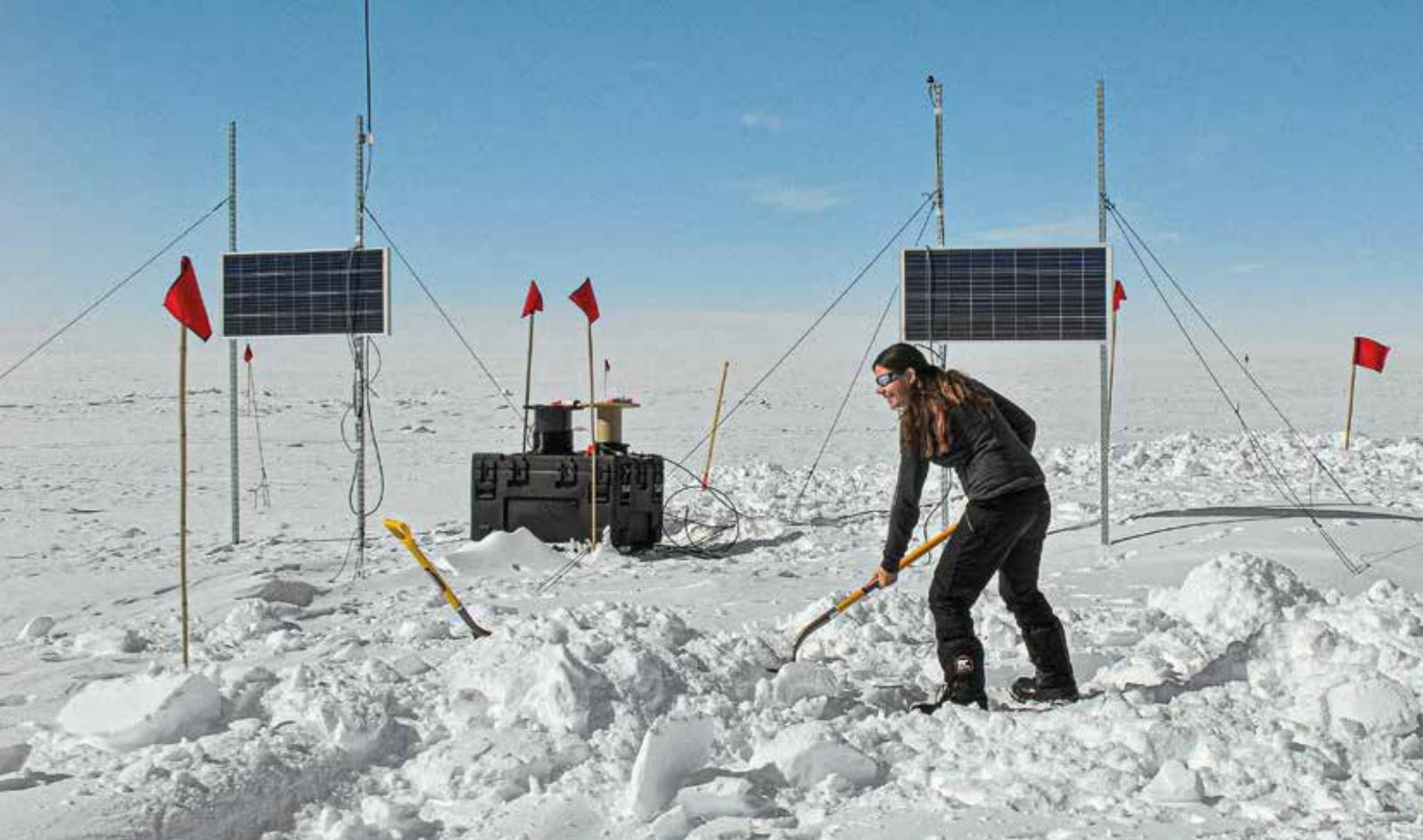
In Greenland's ice sheet, a setup unlike any other in the world will in future be listening for extremely elusive particles from space. The Radio Neutrino Observatory Greenland (RNO-G) is a pioneering project that relies on a new method of detecting very-high-energy cosmic neutrinos using radio antennas, which are being installed on and in the ice.
