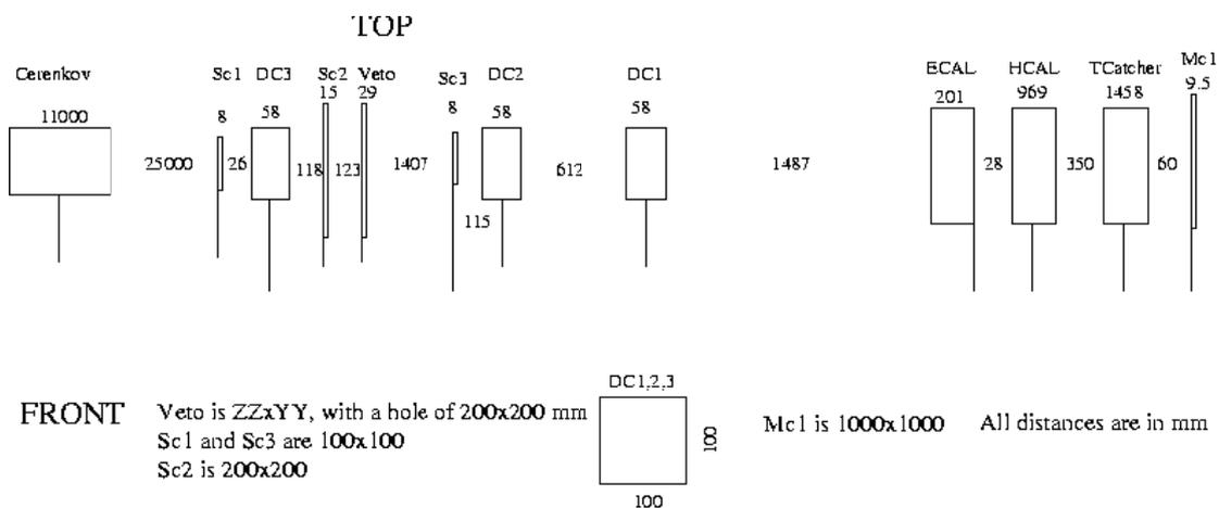
Fig.2: Sketch of the installation for the Calice test beam in the H6B area at the CERN SPS.
