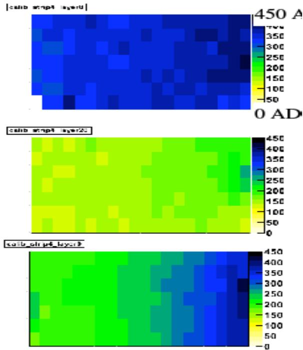
**Figure 4 :** maps of the mip response with ADC output with three typical strips, top : fiber readout with Kuraray scintillator, middle; direct readout with Kuraray scintillator and the bottom : extruded scintillator with fiber readout.
