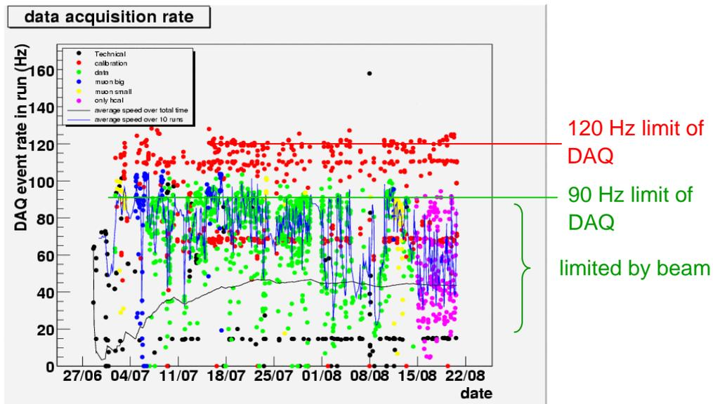
Fig.3: Data acquisition rate for the 2007 Calice test beam at CERN. The average acquisition rate (black line) is ~50 Hz.
