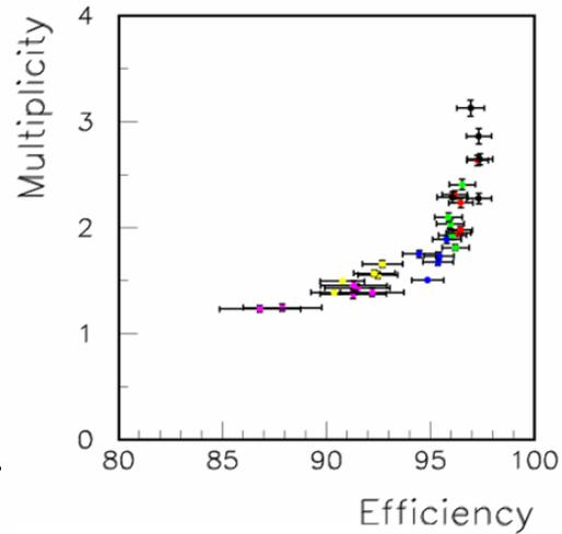
Figure 3 : Pad multiplicity versus efficiency
