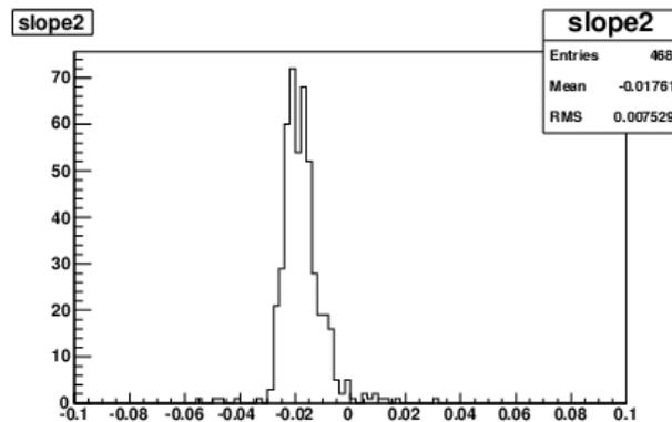
**Figure 2 :** The temperature coefficients distribution for 468 MPPCs in the SCECCAL detector. The average of the coefficients is -1.8%/degree and the r.m.s is 0.8%/degree.
