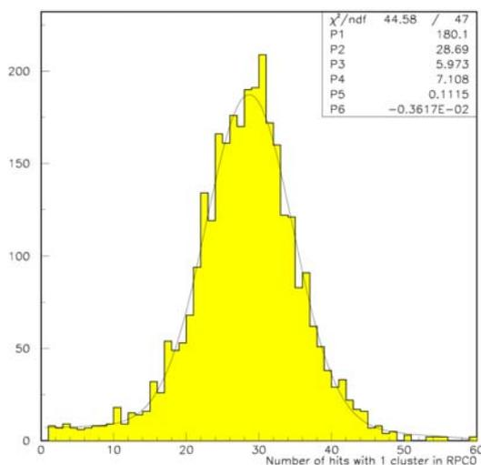
Figure 4. Response to 2 GeV electrons
