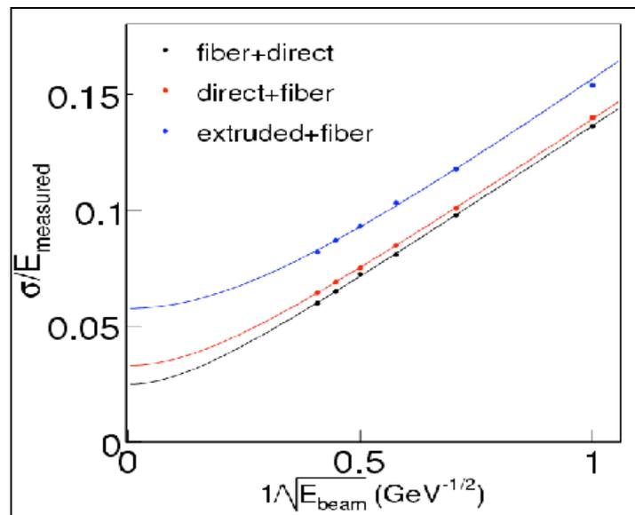
**Figure 3** : the energy resolutions of three types of sub-detector which consists of fiber readout module, direct readout module and extruded scintillator-fibre module.
