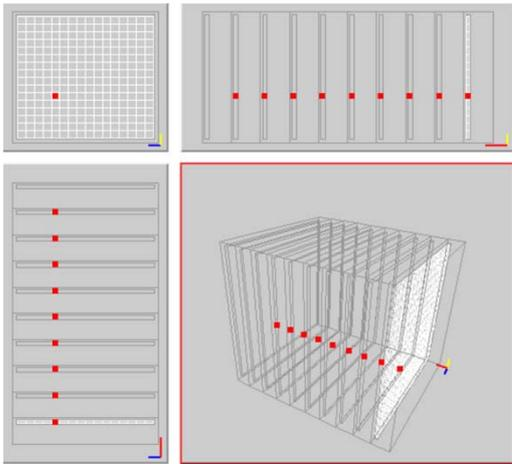
Figure 2. Event display of a muon track
