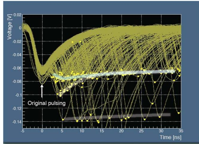
**Figure 1 :** Oscilloscope signals of some single photoelectron equivalent. There are triggered signals and after pulses whose pulse heights are smaller than the previous ones.
