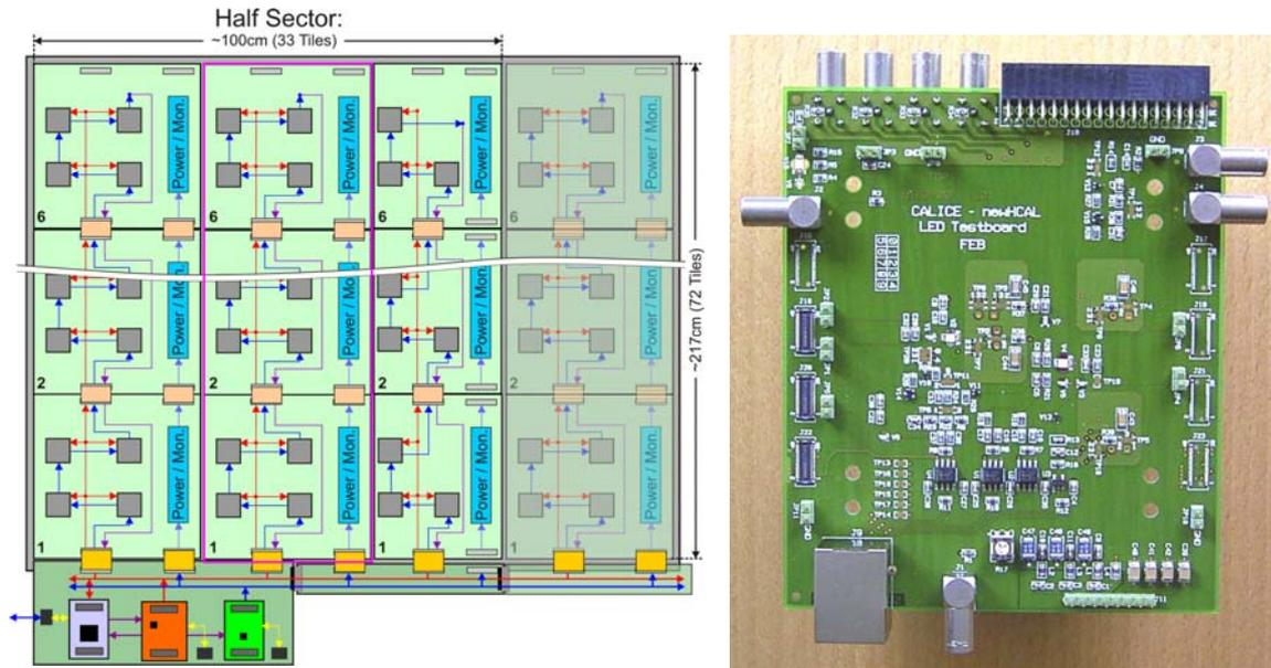
Figure 1 Left: Layout of an HCAL layer with embedded read-out electronics. Right: LED calibration test board.
