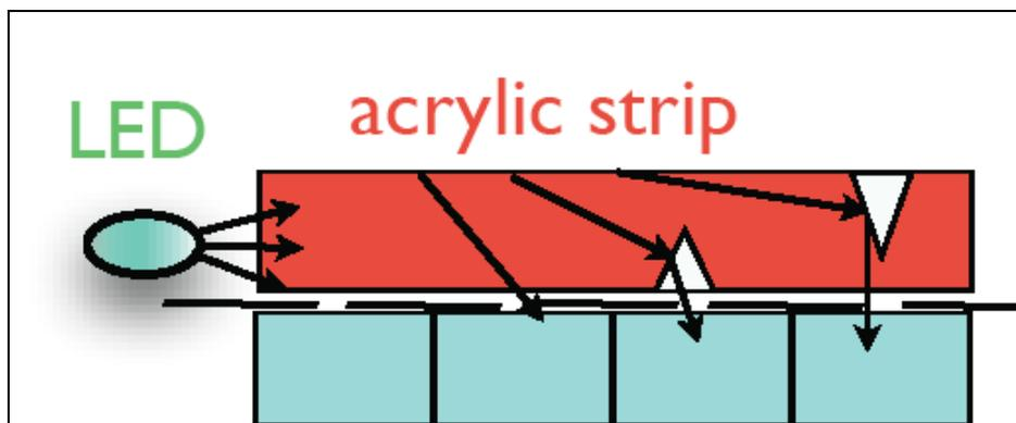
**Figure 5:** a schematic view of the monitoring system. The LED lights are transferred through the acrylic strip and get into each scintillator strips.
