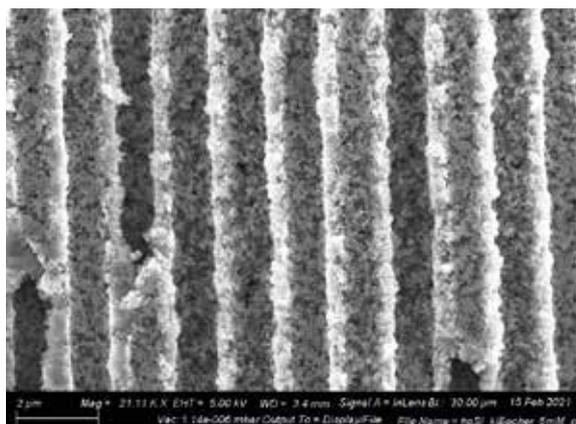
Top view (left) and cross-section (right) of the porous sponge under the electron microscope. The large cylindrical pores have a diameter of around one thousandth of a millimetre. They are separated by nanoporous walls, which are criss-crossed by pores with a diameter of only a few millionths of a millimetre.
