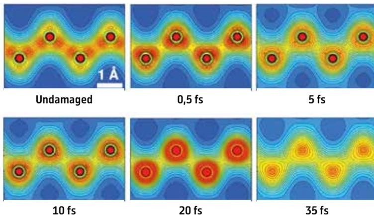
About five quadrillionths of a second (femtoseconds) after the X-ray pulse, the electron distribution around each atom becomes almost uniform in all directions.
