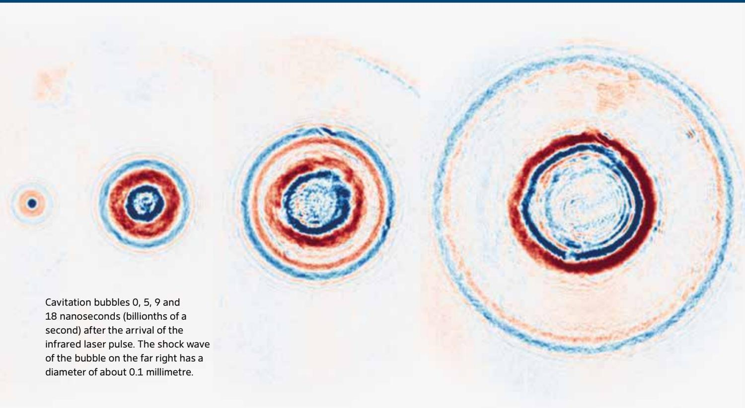
Cavitation bubbles 0, 5, 9 and 18 nanoseconds (billionths of a second) after the arrival of the infrared laser pulse. The shock wave of the bubble on the far right has a diameter of about 0.1 millimetre.
