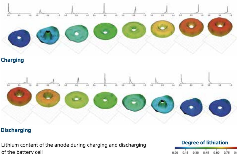
Lithium content of the anode during charging and discharging of the battery cell
