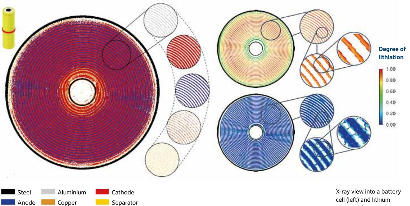
X-ray view into a battery cell (left) and lithium content of its anode (top right) and its cathode (bottom right)
