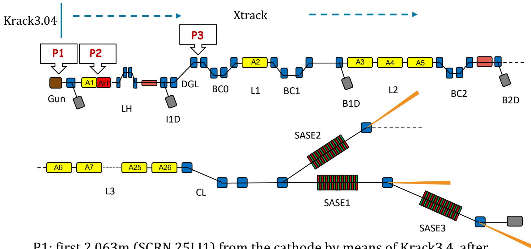
P1: first 2.063m (SCRN.25I.I1) from the cathode by means of Krack3.4, after P1 with Xtrack
