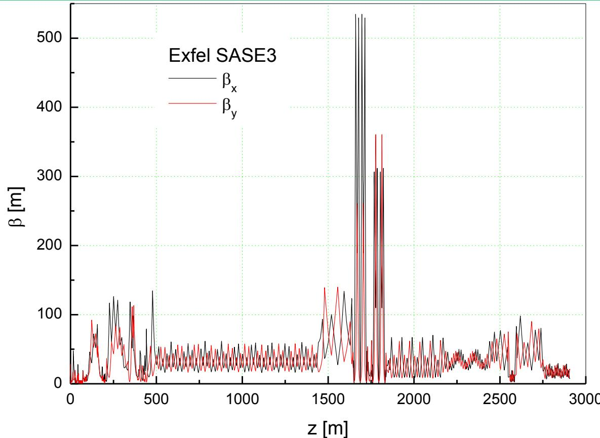
Beta function distribution by using the exact parameters values of the accelerating cavities and bunch compressors (Elegant)
