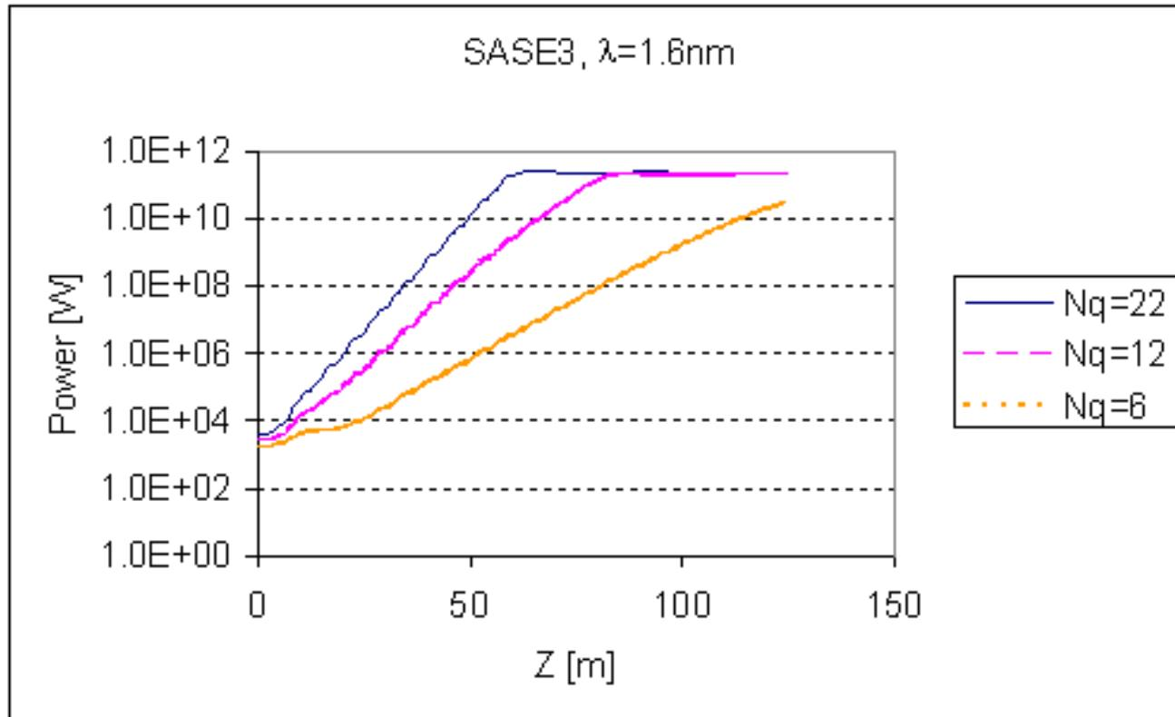
SASE3 FEL GENESIS Steady State Simulation Results; Power growth curves for focusing lattice arrangements with quadrupole magnets number equal to 22, 12 and 6.
