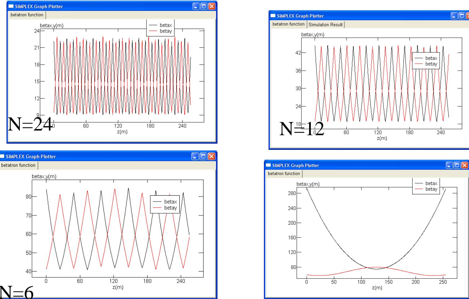
Figure 1. Beta function in x and y direction for XFEL lattices.
