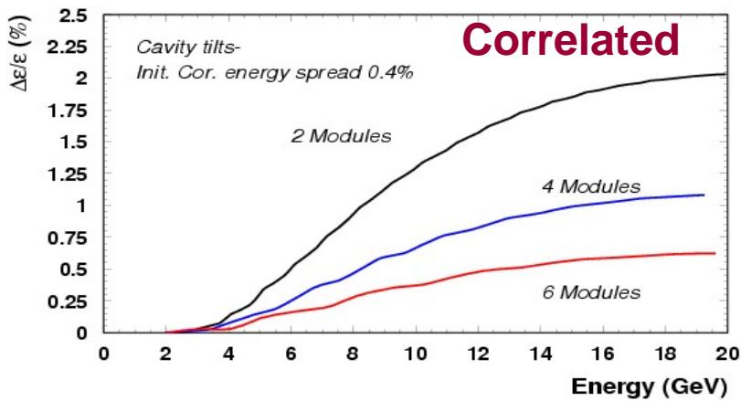
$$\frac{\Delta\epsilon}{\epsilon} = \frac{4}{3} \langle \alpha^2 \rangle \frac{\sigma_0^2 d^2 N_{cav}}{\epsilon_0 L_c \sin \mu} t g^2 \frac{\mu}{2} \frac{\gamma_0}{\Delta\gamma} \ln^3 \frac{\gamma}{\gamma_0}$$
