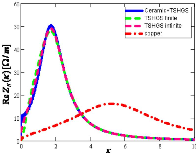
Longitudinal monopole impedance as function of dimensionless wave number  $\kappa = k \cdot s_0$  for several cases of vacuum chamber material:
