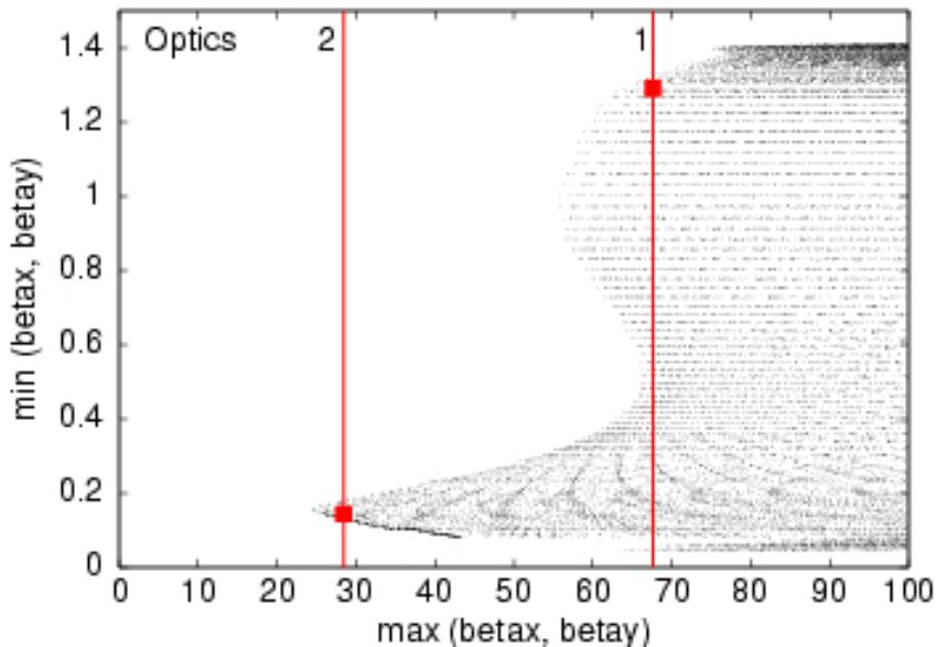
The transition from DBC2 diagnostic section into accelerating module ACC2: Scan over possible strengths of 3 quads downstream of DBC2 FODO => max and min values of  $\beta$ -functions are calculated in the section containing these 3 quads and 8 cavities of ACC2 (no RF focusing).
