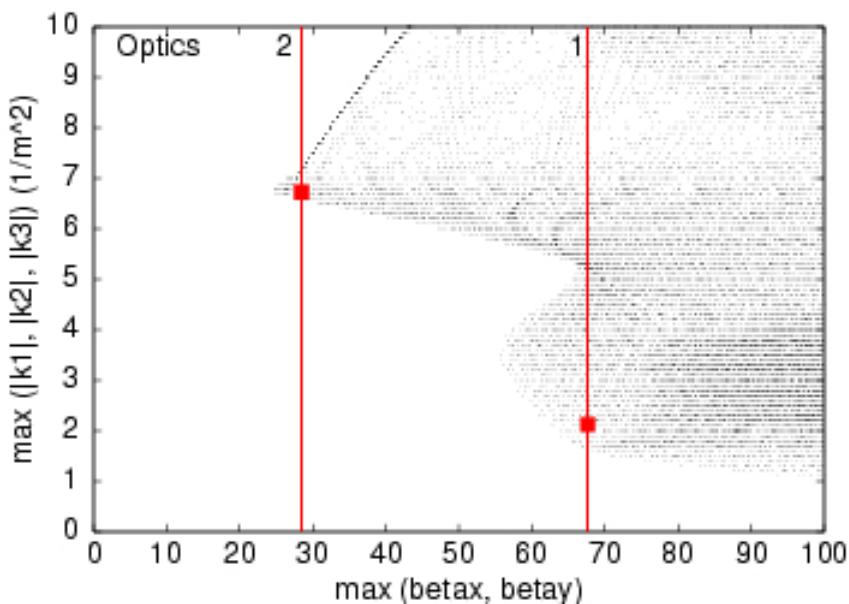
At the reducing of  $\max(\beta_x, \beta_y)$  there are sudden jumps both in maximum of  $\min(\beta_x, \beta_y)$  and in minimum of  $\max(|k_i|)$ ; and there is no continuous transition between two optics.
