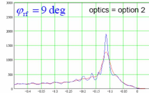
The simulations reproduce the observed double spike structure.
