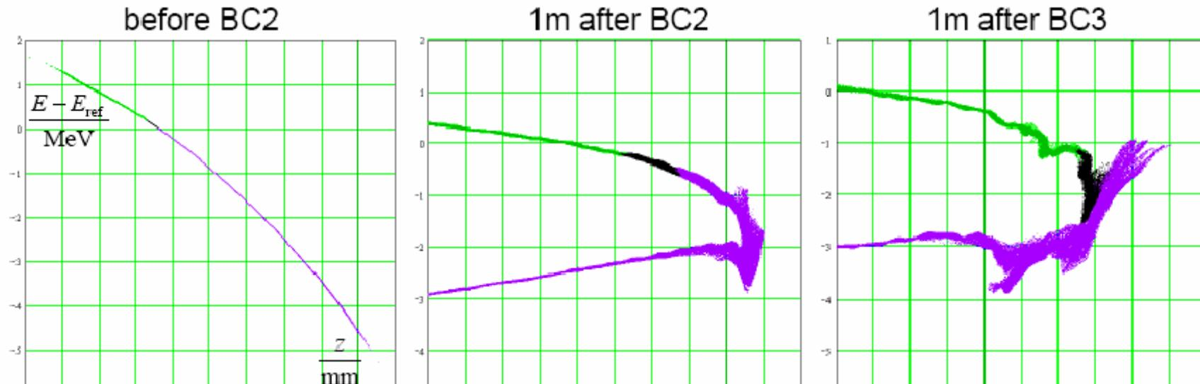
Due to CSR forces a second compression slope in the longitudinal phase space is generated in BC2 and then further compressed in BC3.
