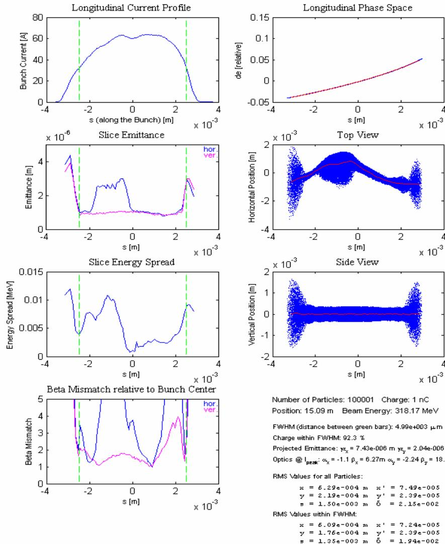
Beam is only compressed in BC3 by keeping ACC1 on crest. The compression chirp is induced by ACC2&3 (40deg off crest).
