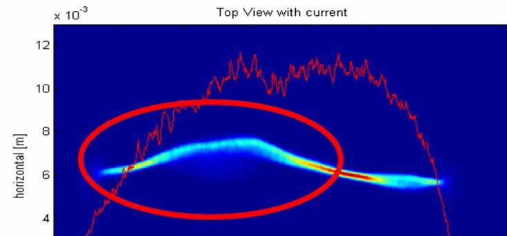
The centroid of the beam is shifted as a result of CSR interaction
