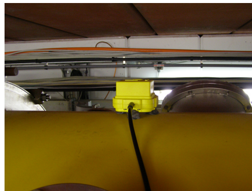
Triaxial sensor on vessel top
