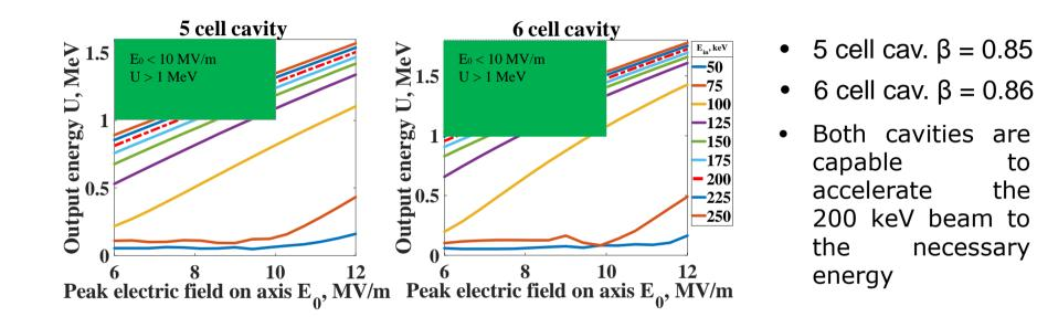
• The six cell cavity is also capable to accelerate the 100 keV beam, which is an advantage over the 5-cell cavity
