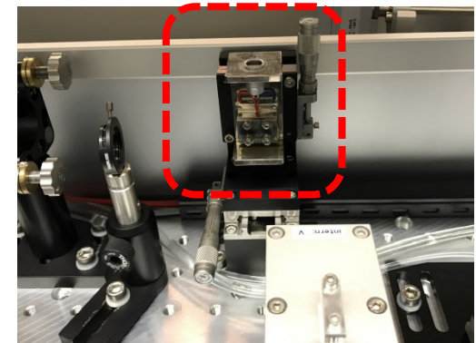
Lyot filter in the regenerative amplifier
