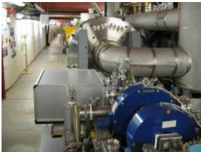
> Normal conducting 1.3 GHz RF gun > Ce 2 Te cathode > Two Nd:YLF based ps photocathode lasers
