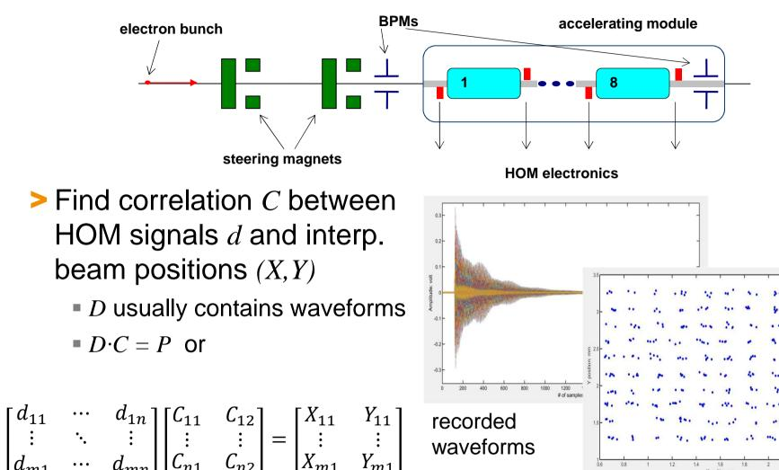
and interpolated beam position in the cavity
