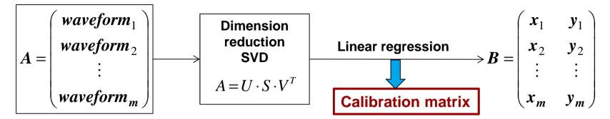
Calibration more complicated than in standard cavity BPMs
