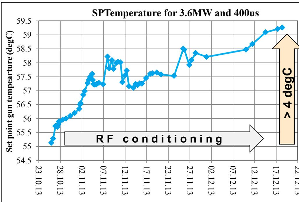
Measurement benchmark: 3.6MW in gun (reflection=4%), 400us, 10Hz
