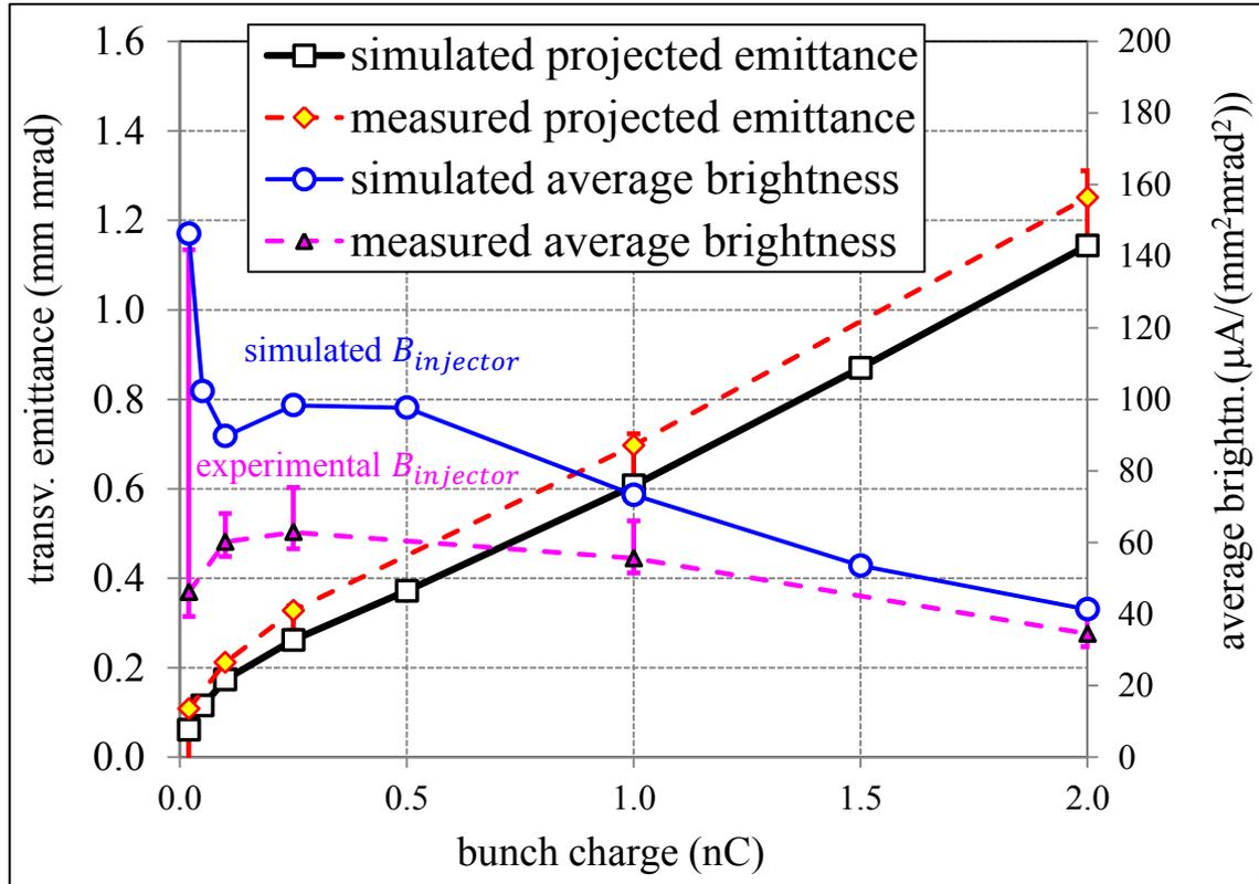
Bunch charge reduction at fixed cathode laser pulse duration  $\rightarrow$  space charge (SC) modification
