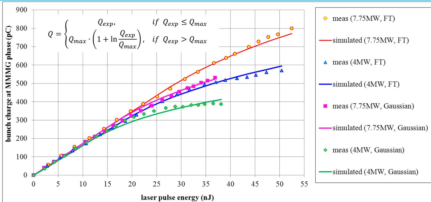
Simultaneous fit of 4 curves using:  $Q_{max}(7.75MW) = Q_{max}(4.0MW) \cdot \frac{E_{cath2} \cdot \sin \varphi_{MMM2}}{E_{cath1} \cdot \sin \varphi_{MMM1}}$
