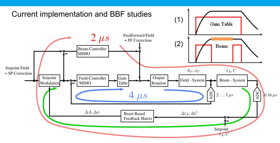
(1) SP Modulation: 4us delay (VME), 2.x us (uTCA)  $\rightarrow$  40fs (rms) after BC2 (2) FF Modulation: 2us delay
