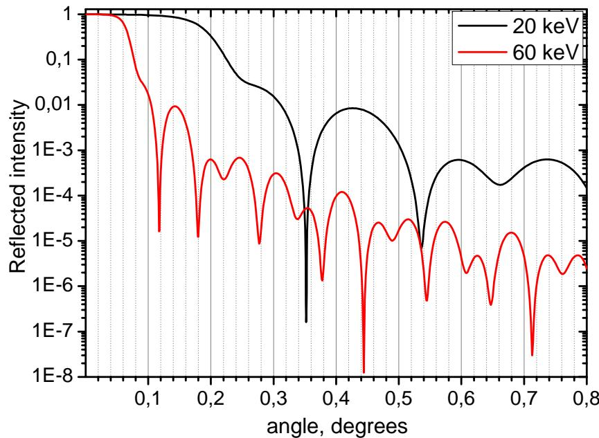
Reflectivity of layer systems can be calculated using Parratt recursive algorithm:
