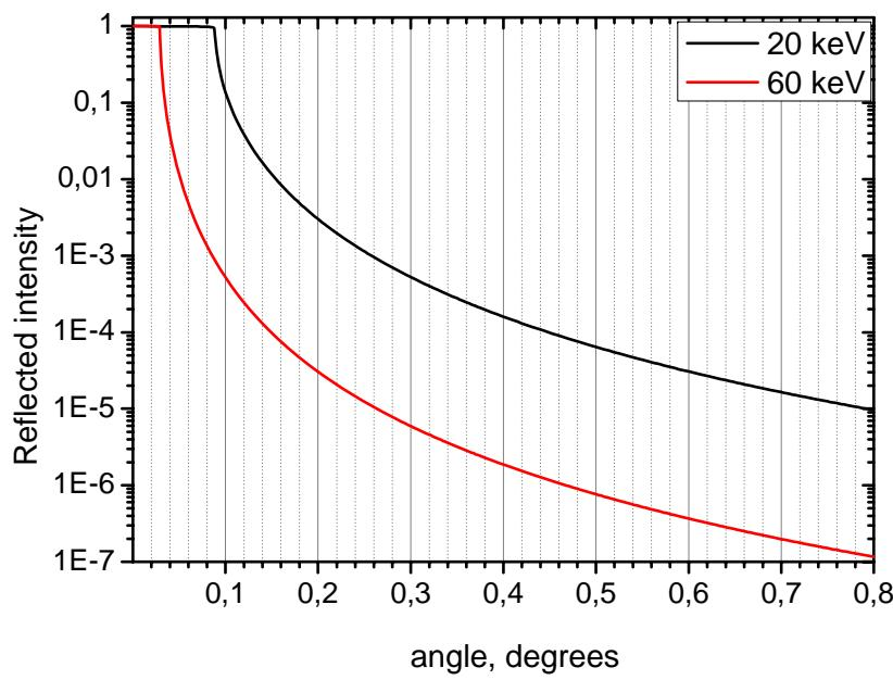
Silicon mirror coated with Rh:  $\alpha_c = 1,30^\circ$
