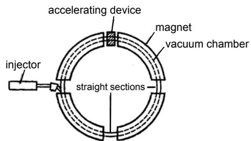
$$\vec{B} \perp \vec{v} \rightarrow F = q v B = m \frac{v^2}{R} \Rightarrow R = \frac{m v}{q B}$$
