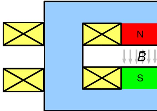
Max.  $B \rightarrow$  max. current  $\rightarrow$  large conductor cables
