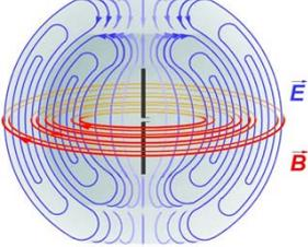
Radiation of an oscillating dipole
