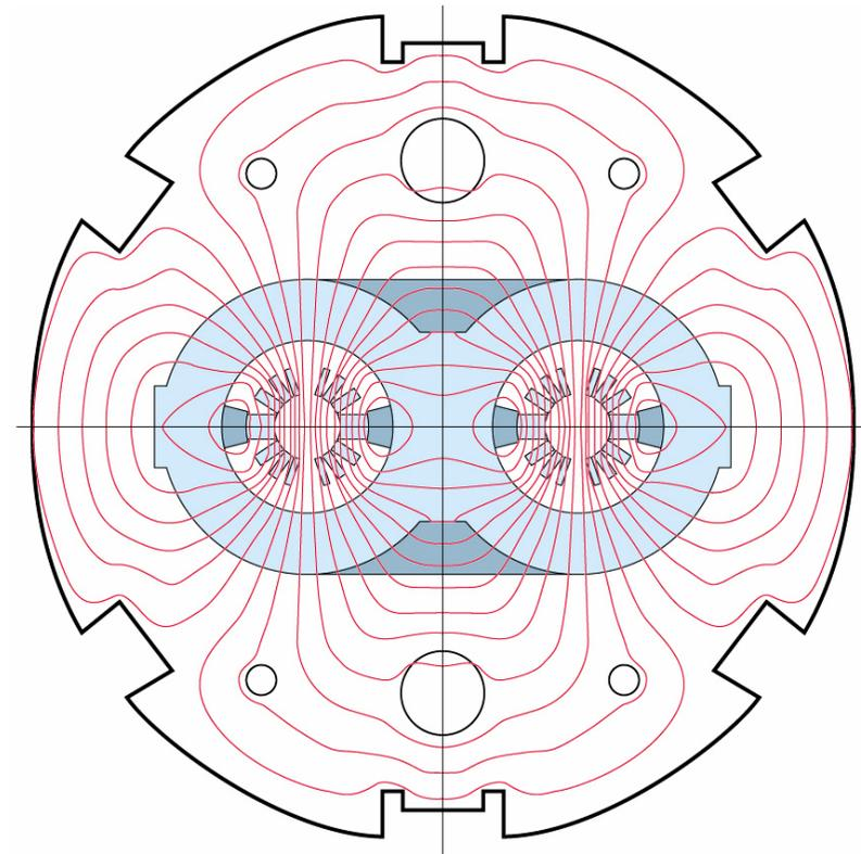
Computed magnetic flux map at  $B_0=10$  Tesla
