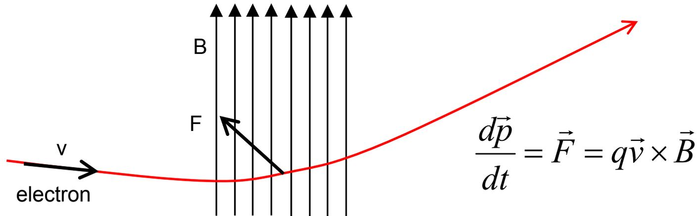
Charged particles when accelerated, emit radiation tangential to the trajectory:
