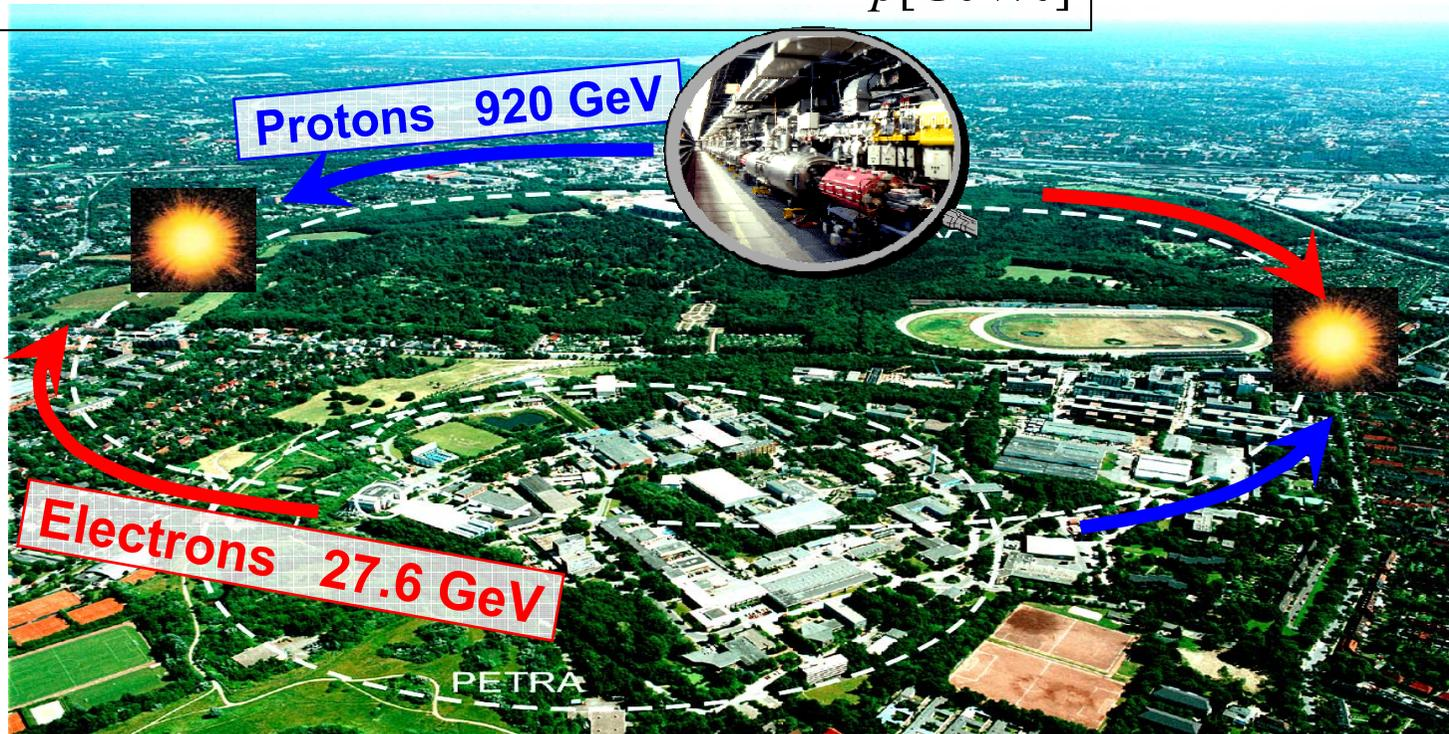
HERA: Hadron-Electron Ring Accelerator, 6.3 km ring, DESY
