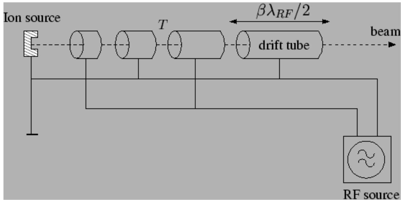
original Wideroe drift-tube principle
