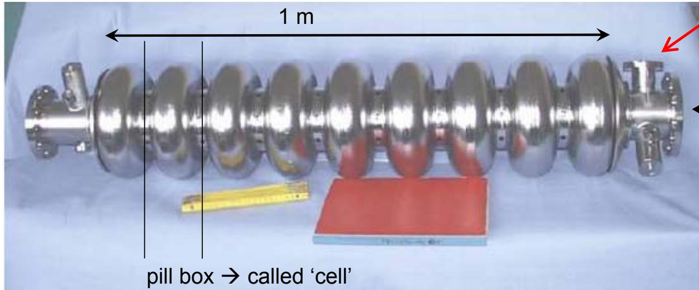
RF input port called 'input coupler' or 'power coupler'
