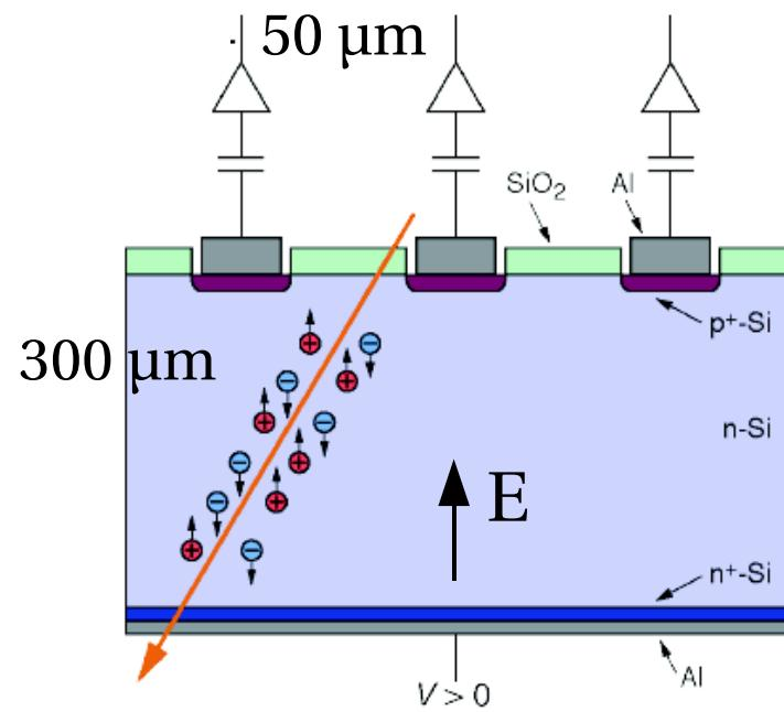
Figure 2.8: Schematic structure of a CMS silicon microstrip sensor.
