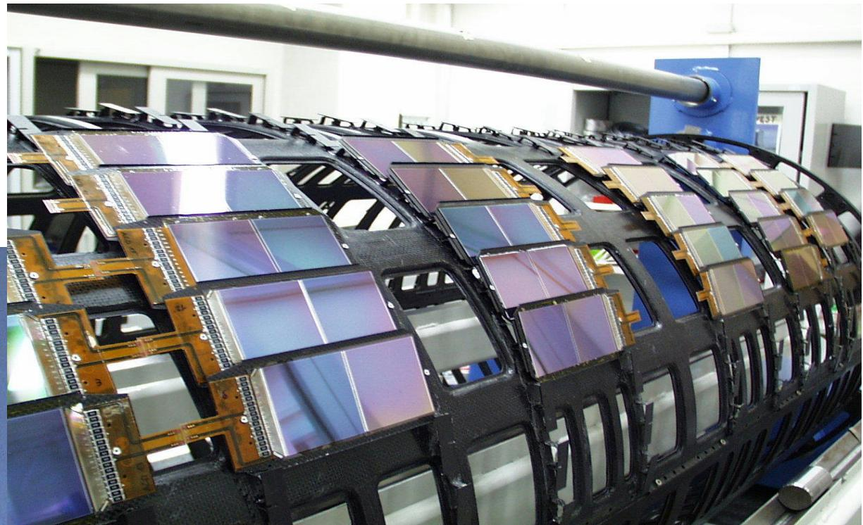
Carbon-fibre support structure.
