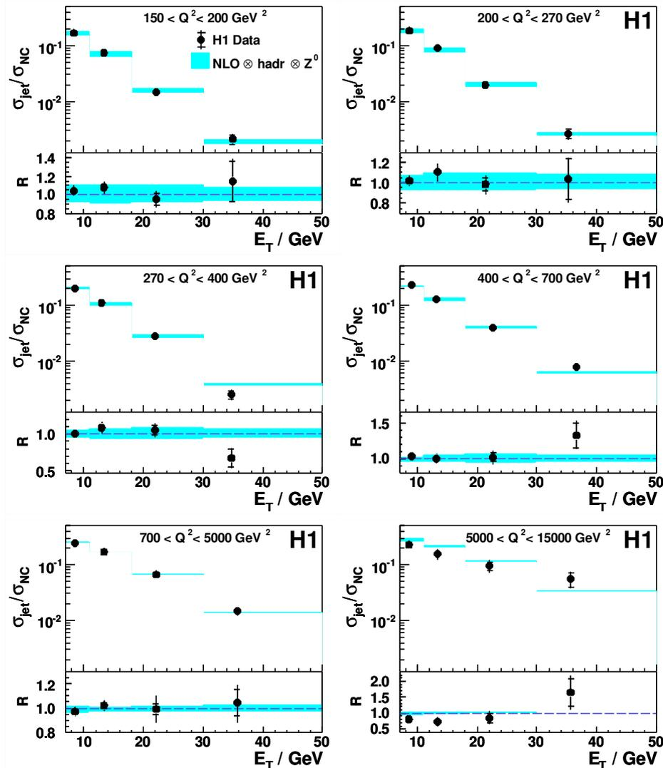
ratio of jet cross section to inclusive cross section has reduced uncertainties
