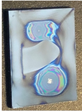
Figure 8: Sample made with 25nm solution with a methanol-polymer ratio 1:1, spun with settings: Step 1, 160RPM , 120s , ramp 6; Step 2, 1000RPM , 10s , ramp 9.
