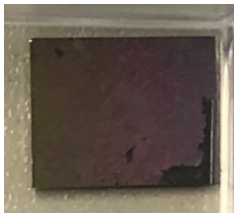
Figure 11: 4\mu\text{m} Polystyrene nanospheres produced by angled Langmuir-Blodgett coating using a 2:8 ratio of methanol to polystyrene solution. Optical microscope image (left) and photo of sample (right)
