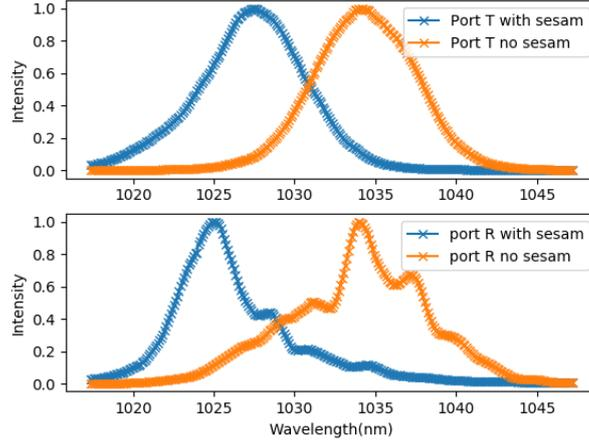
Figure 11: Comparing the spectra of pure NLI with NLI with SESAM at both ports at 460mA.
