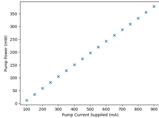
Figure 5: Diode laser's power against the current supplied for the pump.
