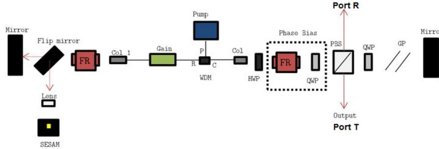
Figure 8: Experimental setup used for mode-locking using nonlinear interferometry. With a flip mirror to connect to SESAM arm for comparative measurements with pure NLI and SESAM with NLI. Col: Collimator, WDM: Wavelength-division multiplexer, R:reflected input of WDM, P: pass input of WDM, C: common output of WDM, HWP: half wave plate, QWP: quarter wave plate, PBS: polarising beam splitter, FR: Faraday rotator, GP: grating pair.
