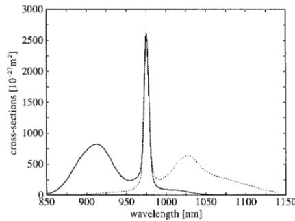
Figure 2: Ytterbium-doped fiber emission (dotted line) and absorption(solid line) spectra. Figure taken from[5].
