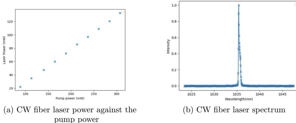
Figure 7: Characterising a continuous wave Yb-doped fiber laser in terms of power and spectrum.
