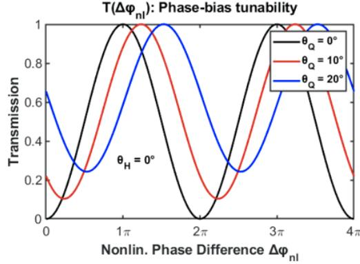
Figure 4: Relationship between pulse intensity and transmission. Adjusting the phase bias will alter the phase difference to find a stable mode-locking point. Figure taken from reference[14].
