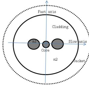
Figure 1: Cross section of a panda fiber, not drawn to scale. The diameter of the core is  $5.5\mu\text{m}$  and the cladding is  $125\mu\text{m}$ . The  $n_1$  is greater than  $n_2$  to maintain the precondition for total internal reflection. The added rods create a fast and slow axis due to increasing or decreasing the relative refractive index across the axis.
