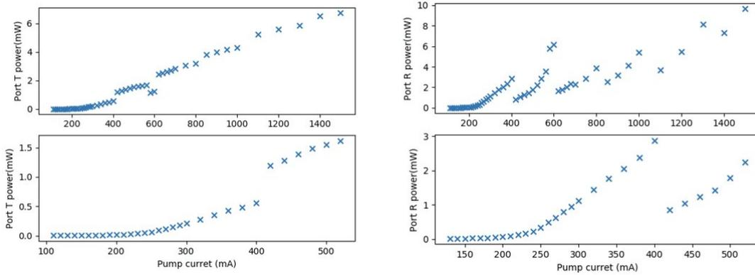
Figure 10: Power curves of the NLI with SESAM laser at both ports.
