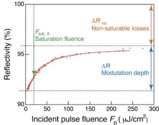
Figure 3: Relationship between fluence/intensity with the reflectivity of a SESAM. This intensity-dependence leads to mode-locking of phases in the laser cavity. Figure taken from reference[13].
