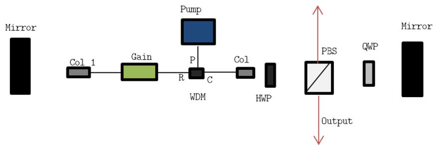
Figure 6: Experimental setup for a CW Yb fiber laser. Col: Collimator, WDM: Wavelength-division multiplexer, R:reflected input of WDM, P: pass input of WDM, C: common output of WDM, HWP: half wave plate, QWP: quarter wave plate, PBS: polarising beam splitter.
