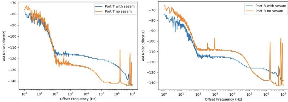
Figure 12: Comparing the AM Noise of pure NLI with NLI with SESAM spectrum at both ports at 460mA.
