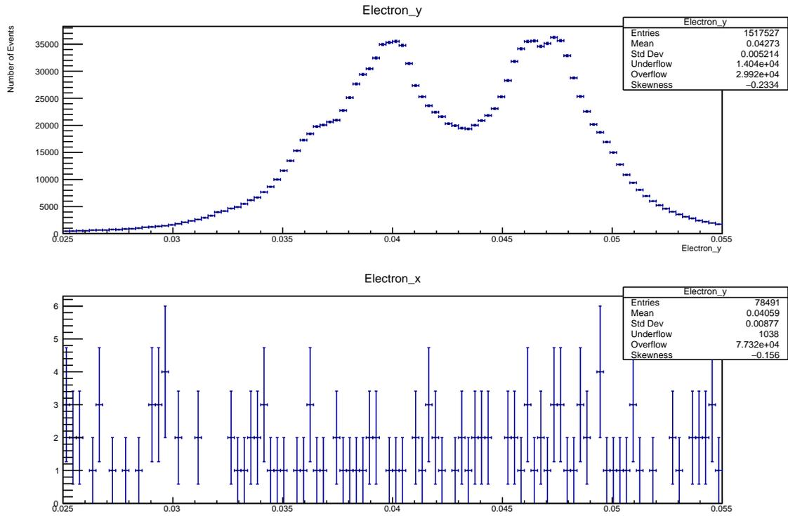
Figure 21:  $y$  point of closest approach to the beamline, in cm. CMS on the top and converted ZEUS below.
