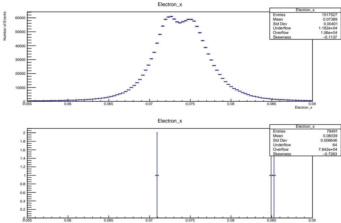
Figure 22:  $x$  point of closest approach to the beamline, in cm. CMS on the top and converted ZEUS below.
