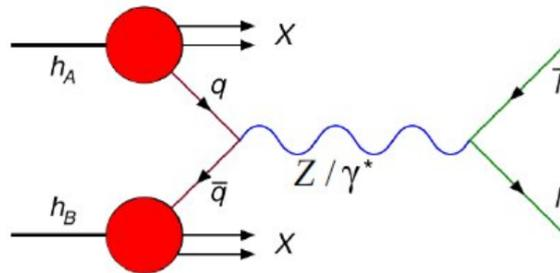
Figure 2: The Feynman diagram for Drell-Yan process.
