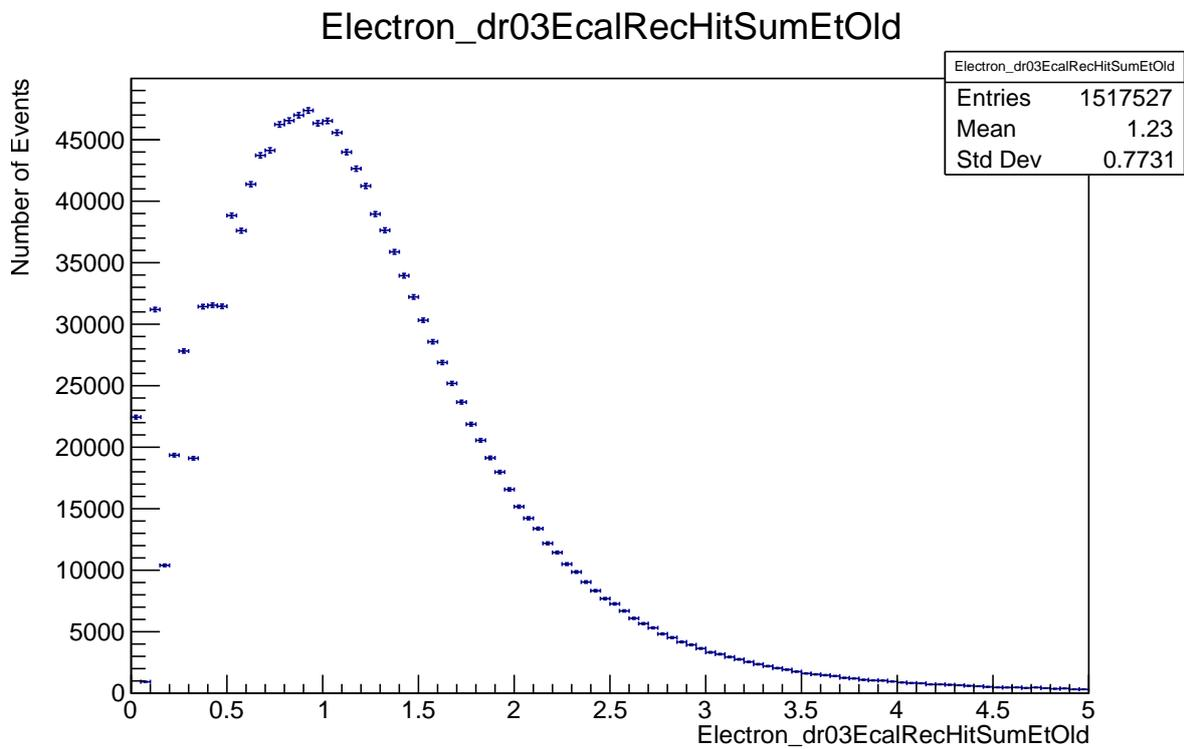
Figure 28: Non-PF Ecal isolation within a delta R cone of 0.3. CMS on the top and converted ZEUS below.
