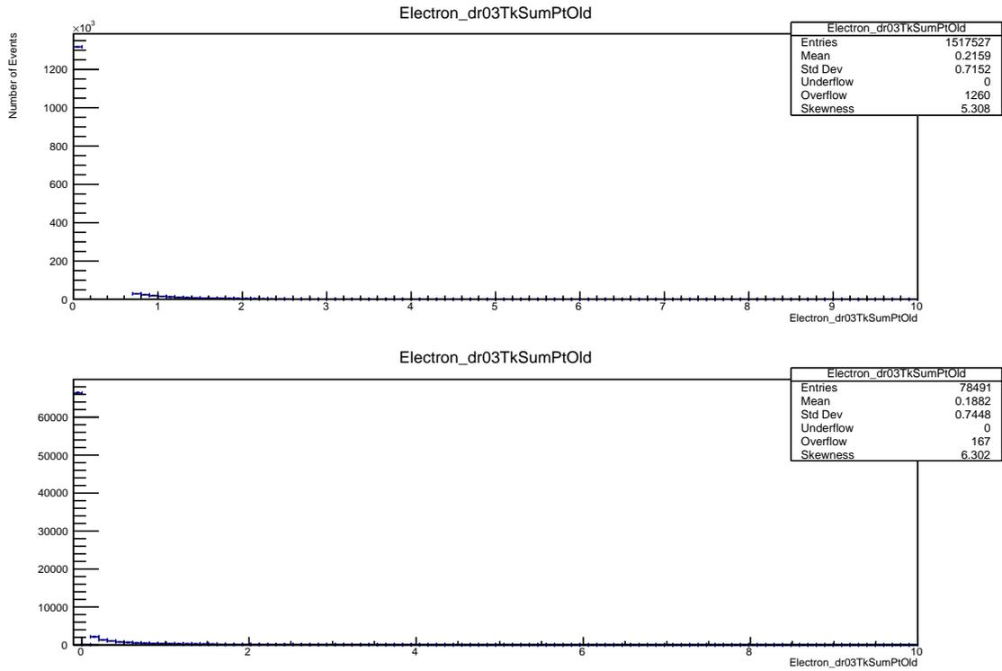
Figure 19: old: Non-PF track isolation within a delta R cone of 0.3. CMS on the top and converted ZEUS below.
