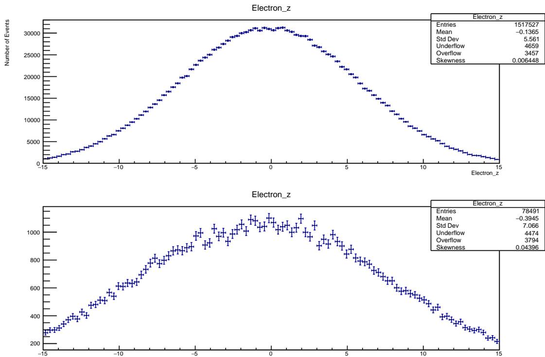
Figure 20:  $z$  point of closest approach to the beamline, in cm. CMS on the top and converted ZEUS below.
