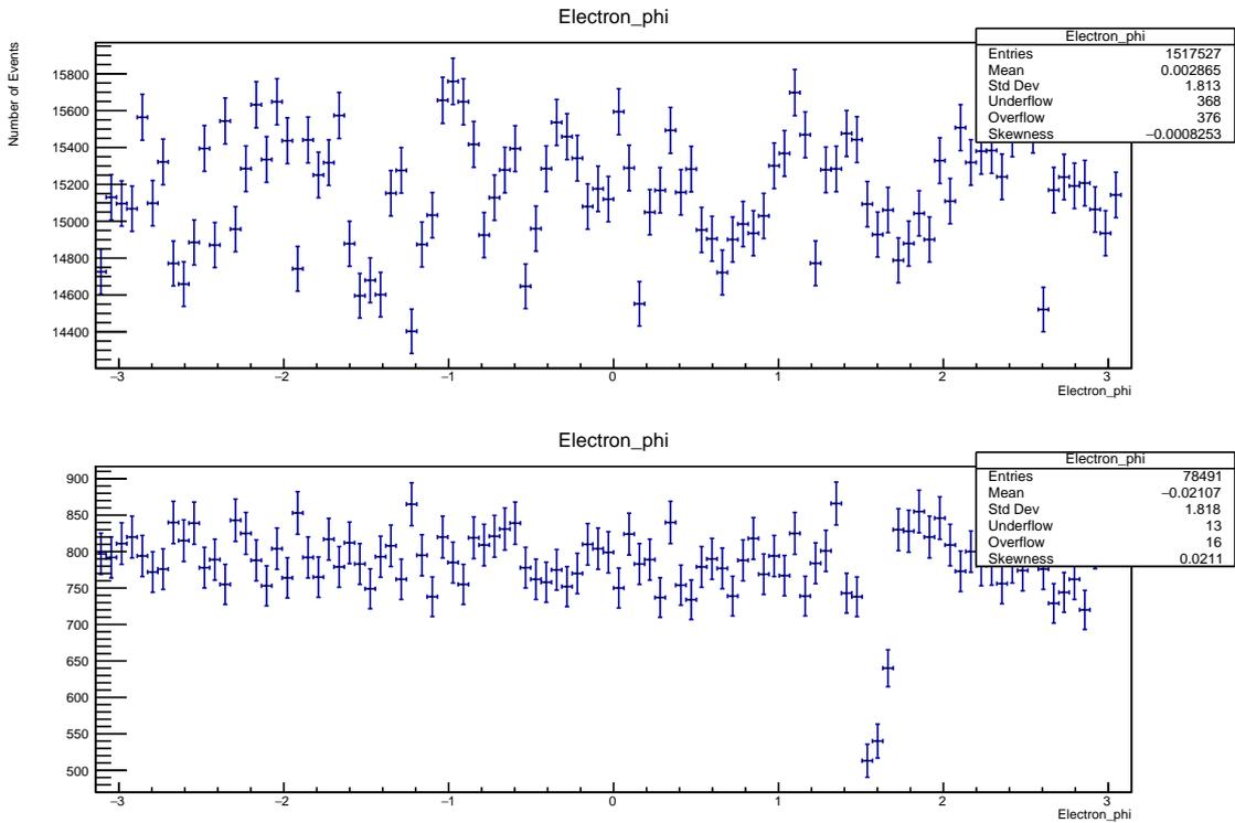
Figure 12: Electron angle  $\phi$ . CMS on the top and converted ZEUS below.
