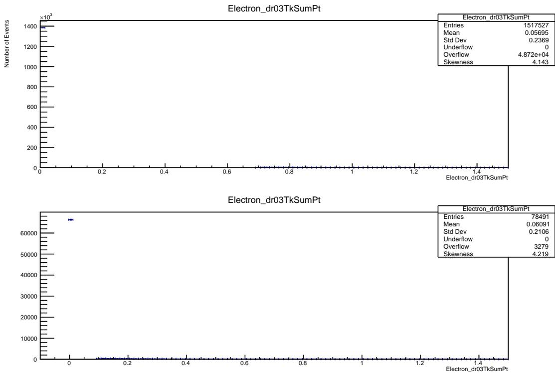
Figure 18: Non-PF track isolation within a delta R cone of 0.3 with electron  $p_T > 35$  GeV. CMS on the top and converted ZEUS below.
