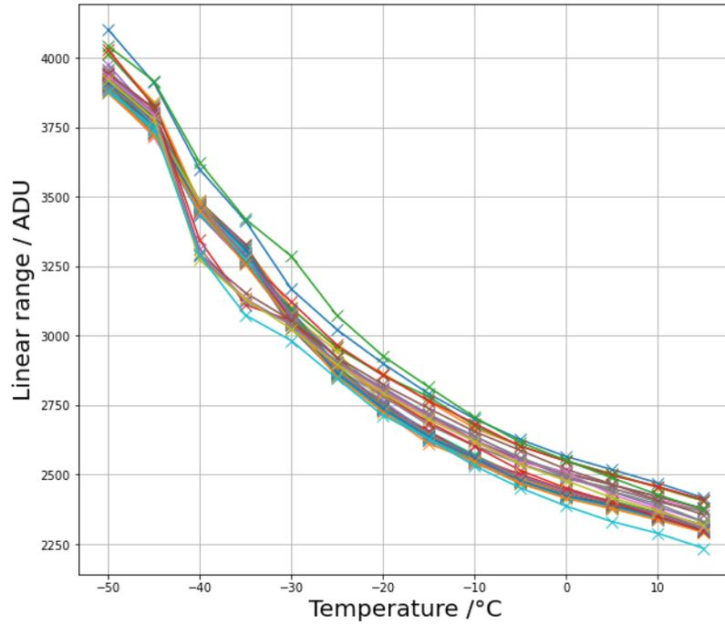
Figure 5: Dependency of the linear range on temperature for all used memory cells
