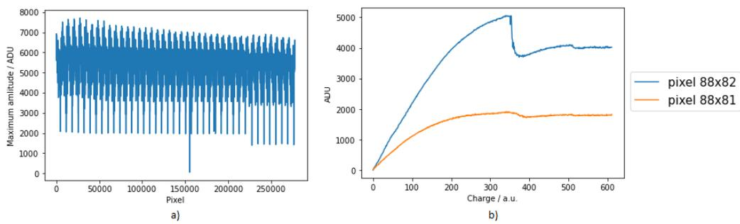
Figure 4: Comparison: a) of the maximum amplitude of the dynamic range scan for the temperature of -45 °C b) of the dynamic range scan for two neighbouring pixels at memory cell 2 for the temperature of -45 °C
