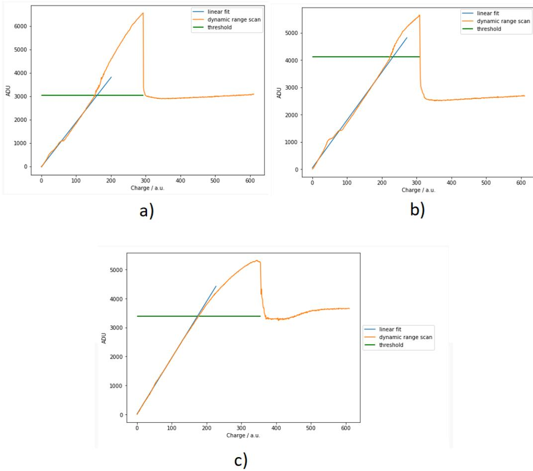
Figure 3: Example of pixels: a) deviation higher than 200, b) correlation coefficient lower than 0.997, c) analysed pixel.
