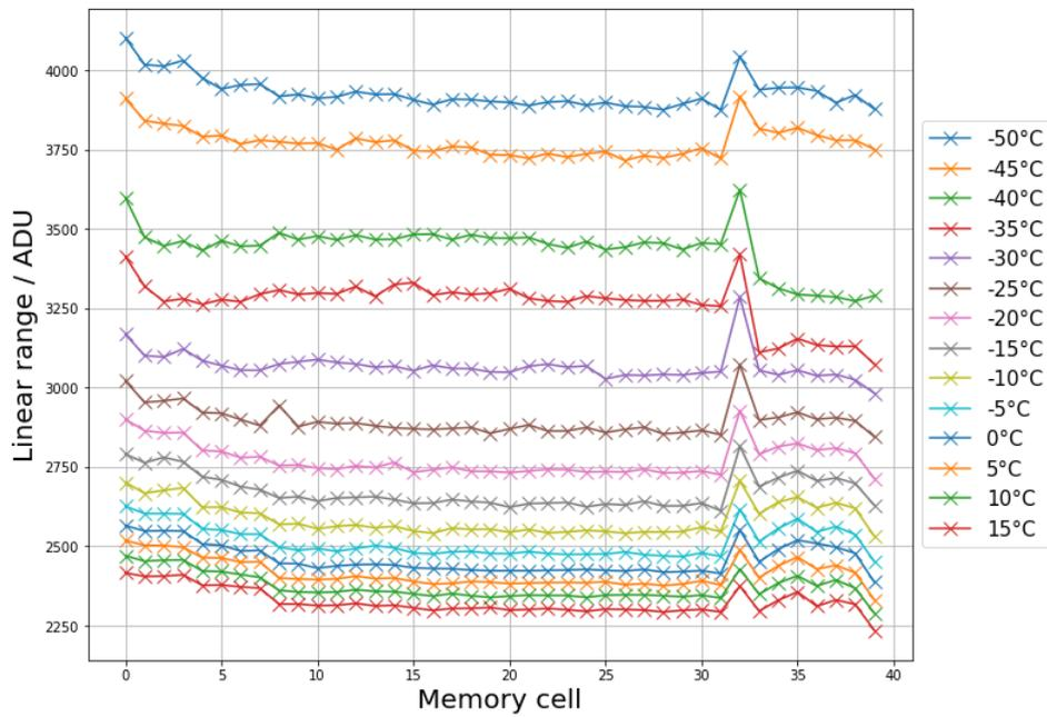
Figure 6: Linear range dependency on memory cell for all of the measured temperatures
