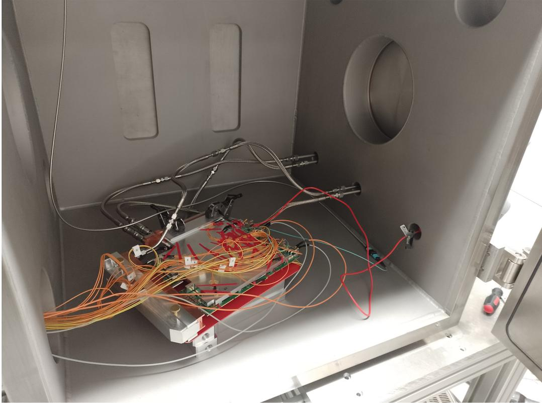
Figure 2: Front-end module, Read-out Board with cooling pipes inside a vacuum chamber
