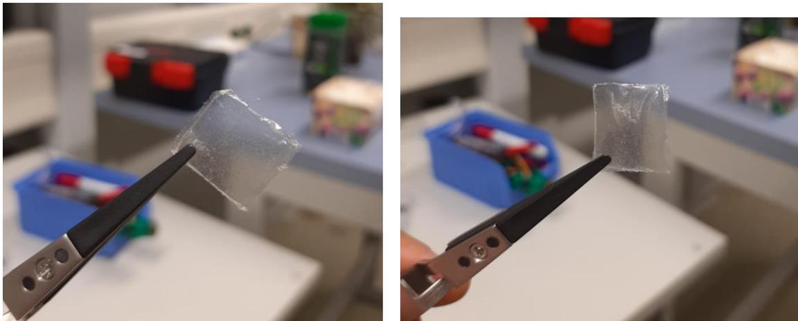
**Figure 10.:** Left image shows the CNF-gel 1000, and on the right is the CNF-gel 400.
