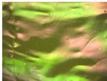
**Figure 24.:** Surface photo of CNF-film sprayed using dropping parameters and 35 pulses at 45°C
