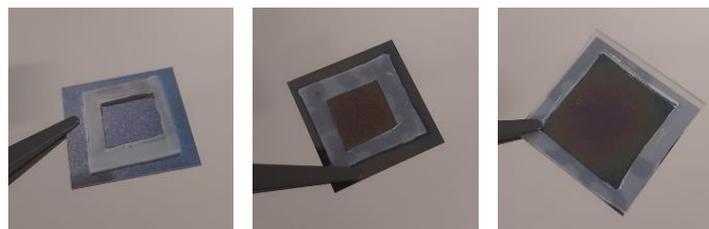
**Figure 17.:** Photos of the silicon wafers sprayed with CNF solution.
