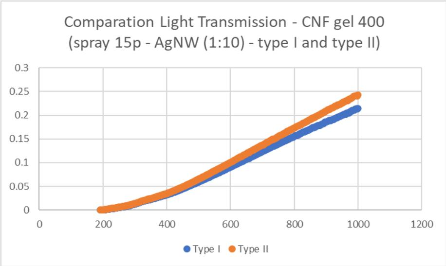
**Figure 33:** Light transmission data from CNF-gel (400) with AgNW ink (type I and type II - concentration 1:10).
