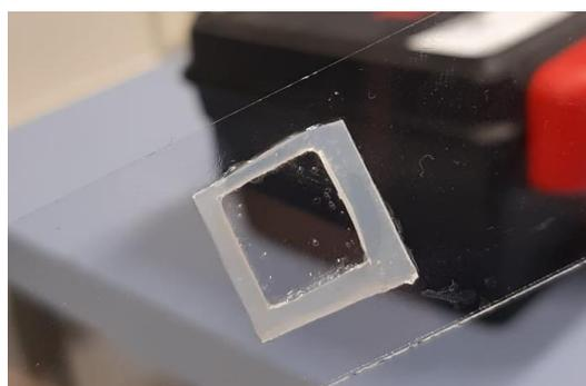
**Figure 22.:** CNF-film sprayed using dropping parameters and 10 pulses at 45°C
