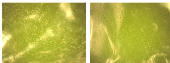
**Figure 36.:** Microscopy image of best sprayed CNF films with AgNW ink Type I (left) and Type II (right) on top.
