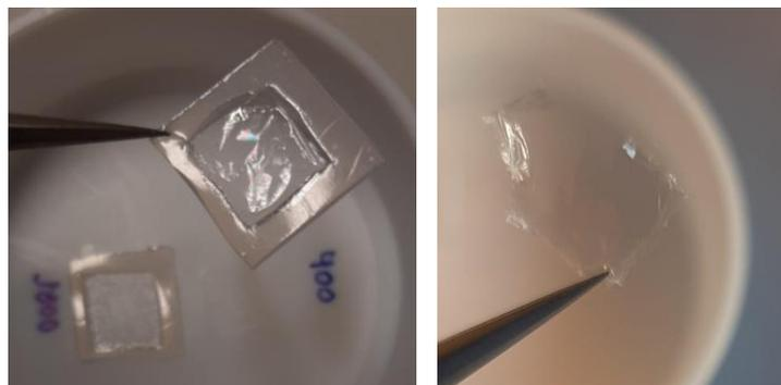
**Figure 15.:** Photos of the film made using the dropping-technique in Teflon
