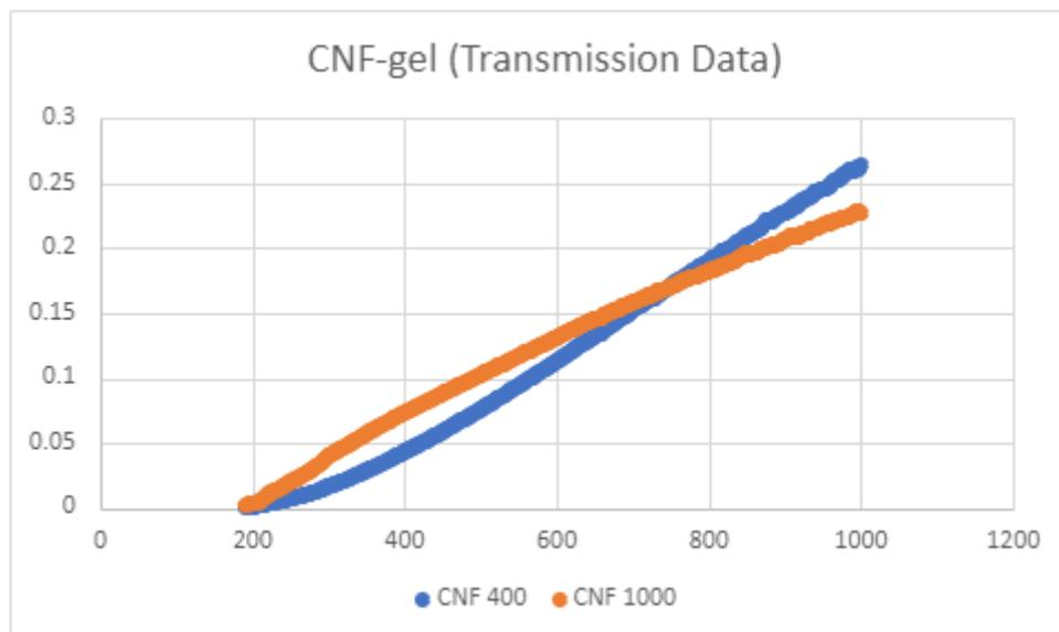
**Figure 11.:** Transmission data of CFN-gel films.
