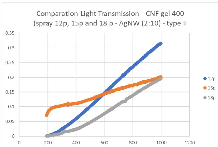
**Figure 35:** Light transmission data from CNF-gel (400) with AgNW ink (type II - concentration 2:10).
