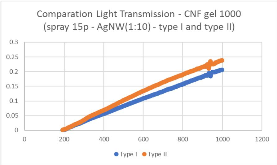
**Figure 34:** Light transmission data from CNF-gel (1000) with AgNW ink (type I and type II - concentration 1:10).
