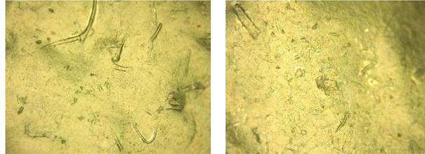
**Figure 31.:** Surface of CNF-gel film (1000) sprayed with AgNW ink type I (right) and type II (left).
