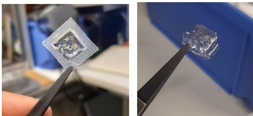
**Figure 21.:** CNF-film sprayed using dropping parameters and 30 pulses.
