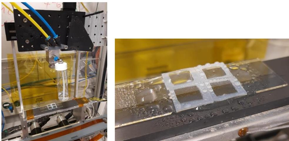
**Figure 27.:** Photo of the spray setup and the frames filled with CNF solution.
