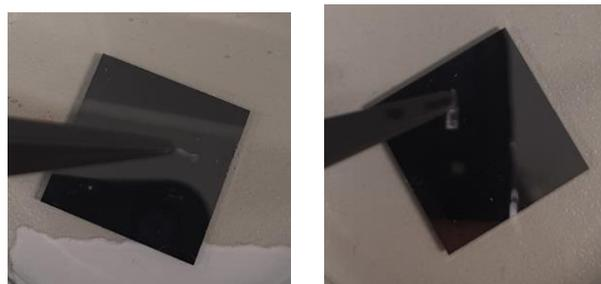
**Figure 18.:** The first photo shows 20 spray pulses (p), and the second shows 100p.
