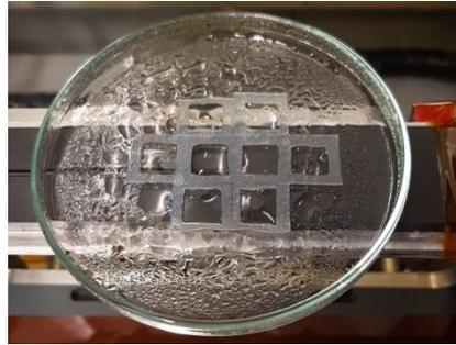
**Figure 26.:** Photo of the amount of solution that spreads due to the focus of the nozzle
