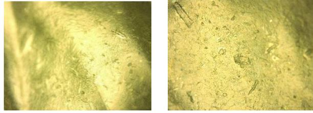
**Figure 31.:** Surface of CNF-gel film (400) sprayed with AgNW ink type I (right) and type II (left).
