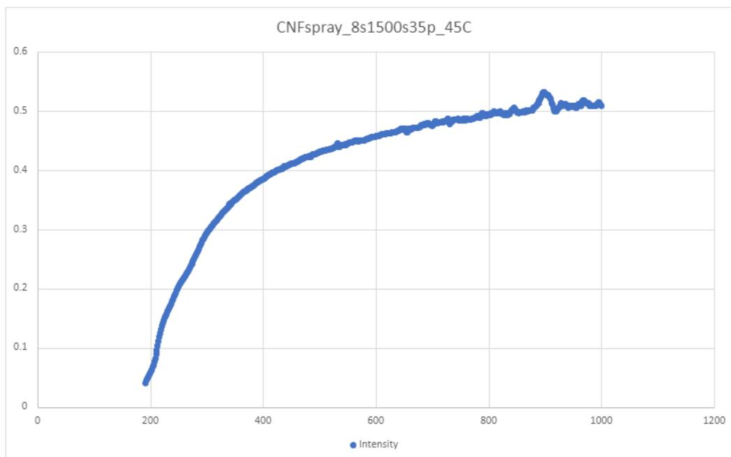
**Figure 25.:** Light transmission of CNF-film sprayed using dropping parameters and 35 pulses at 45°C
