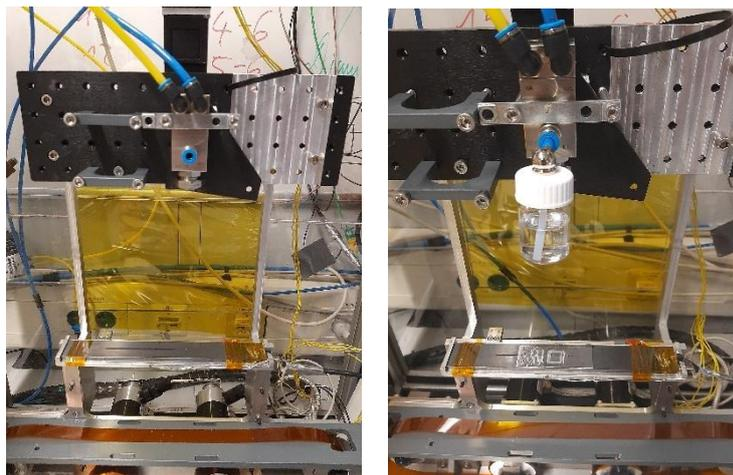
**Figure 6.:** Spray setup used at the synchrotron beamline P03 at DESY.<sup>[2]</sup>
