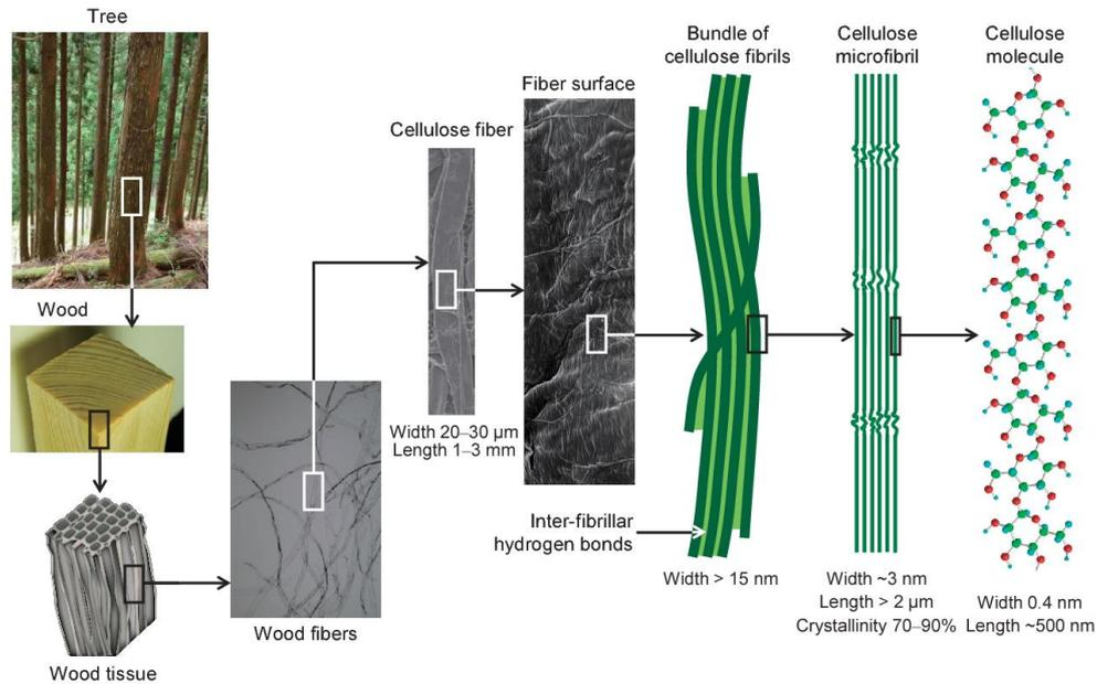
**Figure 1.:** The hierarchical structure of wood. Adapted from A. Isogai, T. Saito and H. Fukuzumi, *Nanoscale*, 3, 71–85, 2011.
