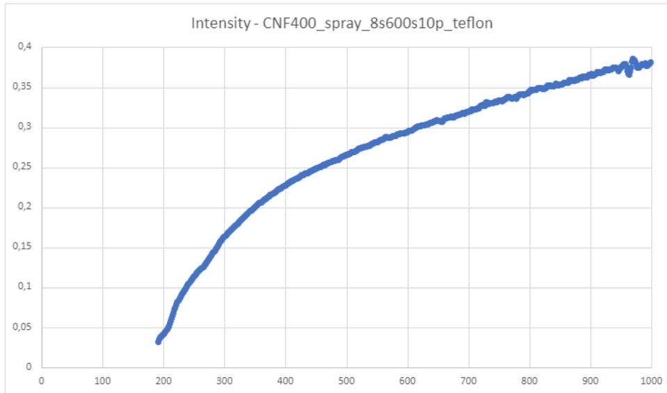
**Figure 20.:** The light transmission data of the CNF-film sprayed on Teflon using 10 pulses.
