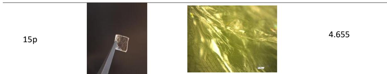
The solvent test results proved that water makes the film less transparent, so it is important to avoid using water to remove films from the substrate. Therefore, to discover how many layers are necessary to take off the films sprayed on the glass without water, the CNF solution was sprayed using the same parameters, but with 30 spray pulses. It was possible to remove the films in air easily, photos of the films are below (Figure 21.).
