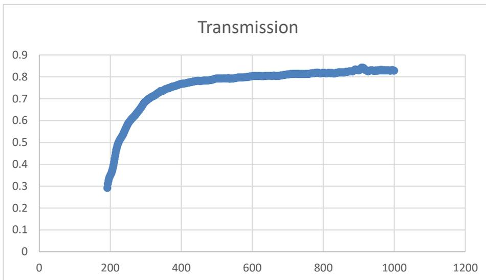
**Figure 30.:** Light transmission of the CNF films produced.
