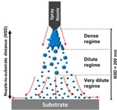
**Figure 5.:** Schematic of the spray or atomization process.<sup>[2]</sup>
