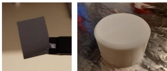
**Figure 7.:** Photos of the used substrate materials: Silicon wafer (left image) and Teflon (right image).
