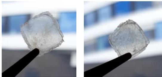
**Figure 32:** Photo of the CNF-gel 400 films after 15p (right) and 18p (left) of AgNW ink (type II).
