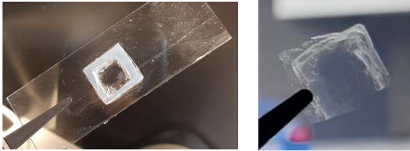
**Figure 23.:** CNF-film sprayed using dropping parameters and 35 pulses at 45°C
