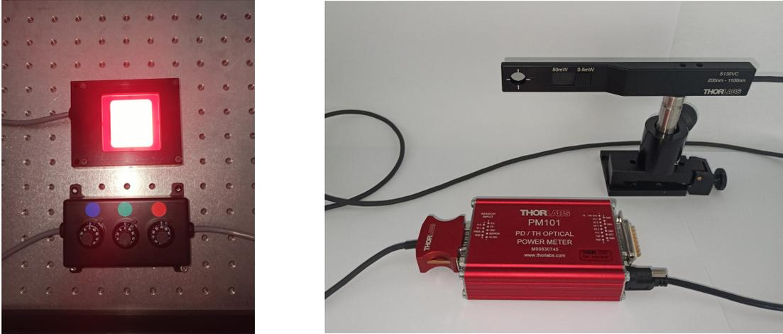
(a) LED light source and control (b) Photodiode used to measure light irradiance and PM 101 device.
