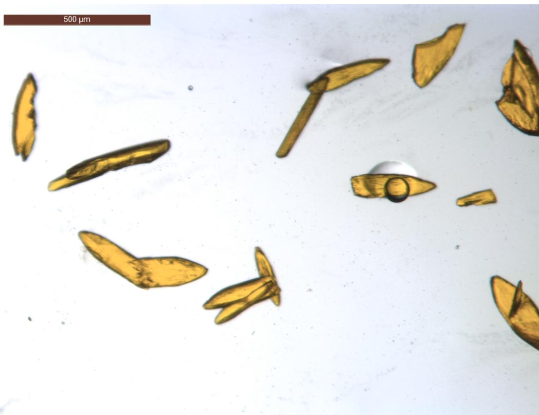
Figure 1: Microphotography of PyDMA18 crystals crystallized with use of pyridine
