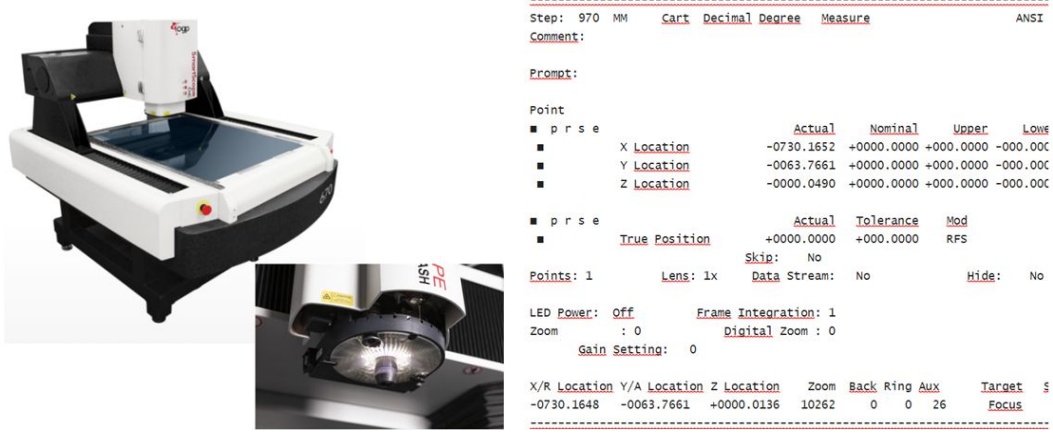
Figure 4: The layout of Smartscope used for flatness measurements [3] and a typical result of a measurement.
