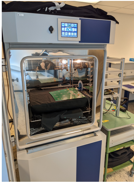
Figure 7: Climate chamber
