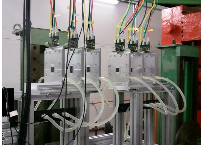
Figure 6: The DATURA telescope installed at the DESY testbeam area. The telescope mechanics and the sensor aluminum enclosure. [1]
