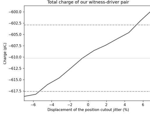
Figure 12: Determination of the cut-out position jitter that relates to the experimental charge jitter downstream bunch-pair generation. The originally to the sub-percent-level stable total charge of the bunch pair (gray) develops a remarkable 1.2% charge jitter (dashed) after bunch separation via collimation in a dispersive section. This bunch charge jitter can be understood as a beam orbit jitter at the location of the collimators and relates to a 5.3% displacement of the cut-out position as a fraction of the cut-out width.
