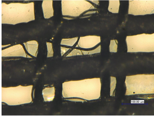
Figure 5: Spray Deposition of a CNF (5:1) layer. Coverage is still weak, even with this higher concentration.
