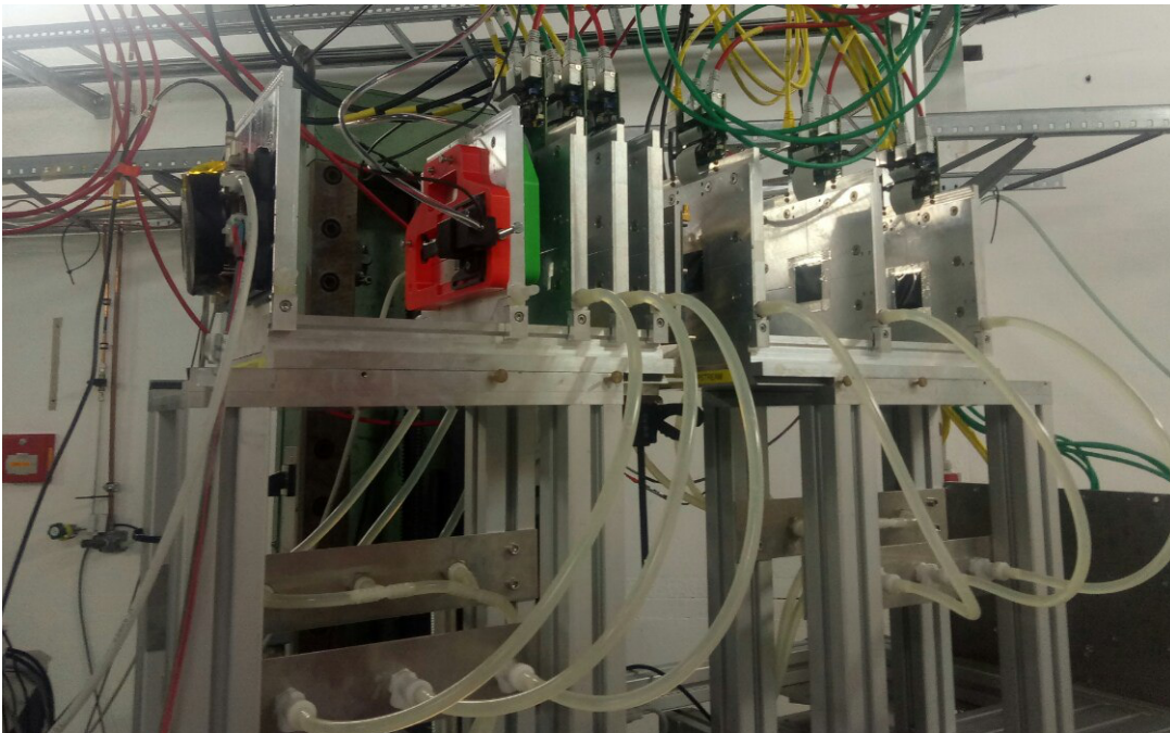
Figure 2: The DURANTA beam telescope with its sensor planes on aluminium rails.
