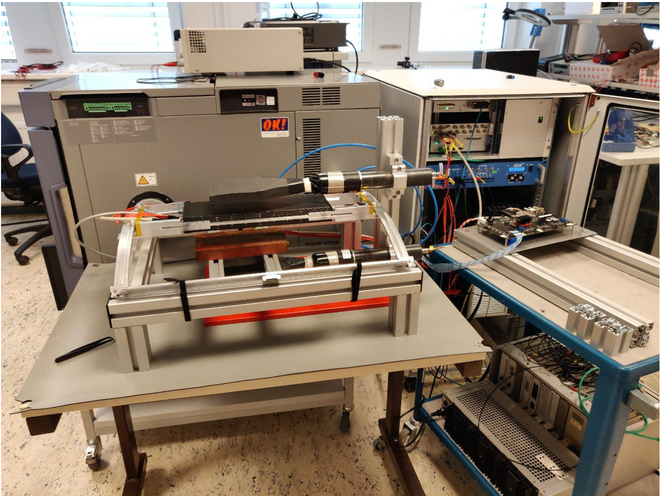
Figure 5.4: Setup in the eLab. The telescope and a lead block are placed between two scintillators; photomultipliers are powered with 1150 V; the DAQ board can be seen on the table on the right, and the Trigger Logic Unit, or TLU, is the blue module on the right.
