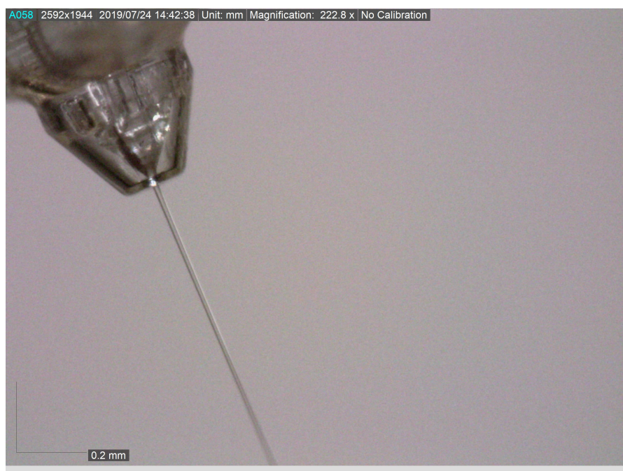
Figure 4: Image of a jet capture with Dinocam at magnification 222.8x, illumination from the camera alone.
