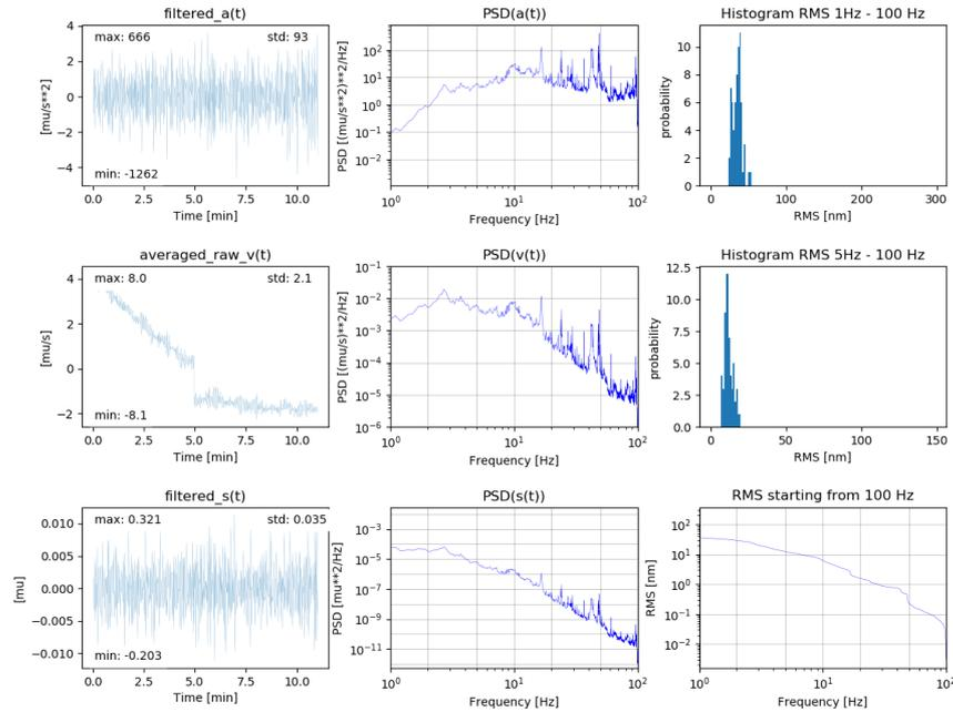
**Figure 2.2:** Vertical vibrations data from the SPB Optics hutch.
