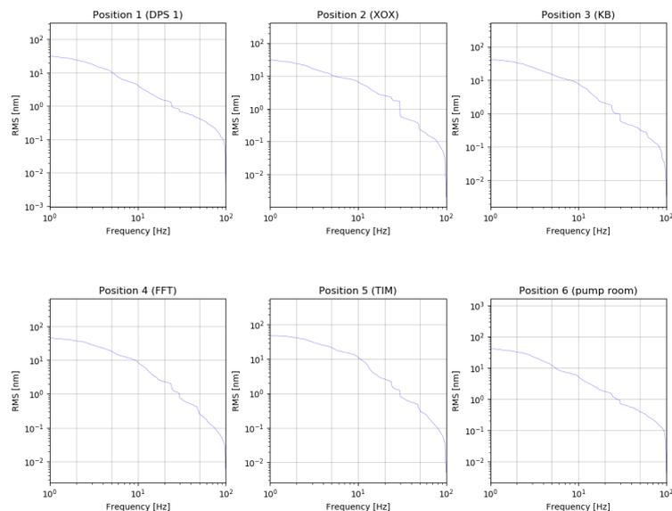
**Figure 2.14:** Vertical RMSs of different measurements depending on the position inside SCS-exp.
