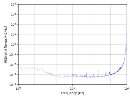
**Figure 2.21:** E-W PSD measured before the left anchor (more damped).
