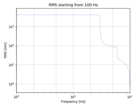
**Figure 2.12:** z RMS with seismometer touching pump from SCS-exp.
