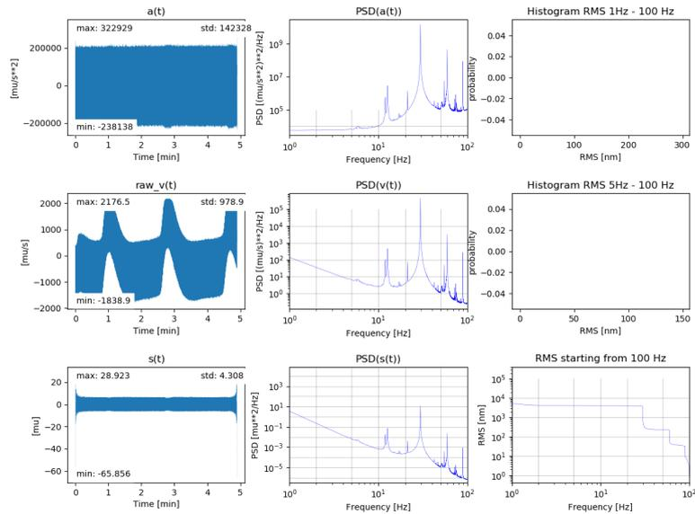
**Figure 2.6:** Measurement in the horizontal direction with the seismometer *touching* a pump from SCS-exp.
