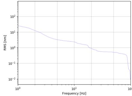
**Figure 2.27:** E-W RMS with seismometer below table support for the beam pipe inside HED-exp.
