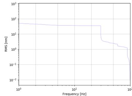
**Figure 2.16:** z RMS with seismometer not touching pipe in SCS-exp.
