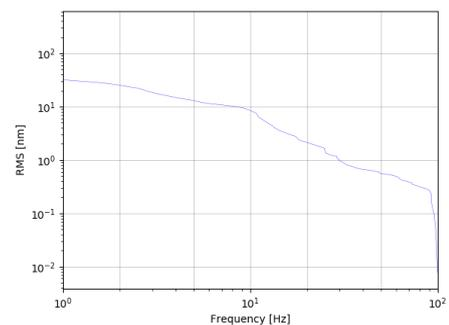
**Figure 2.26:** z RMS with seismometer on top of table support for the beam pipe inside HED-exp.
