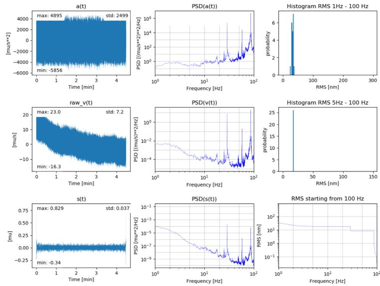
**Figure 2.7:** Measurement in the horizontal direction with the seismometer *next to* a pump from MID-opt.
