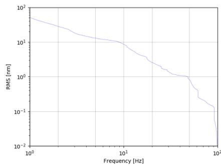
**Figure 2.23:** z RMS with seismometer below optics support inside HED-opt.
