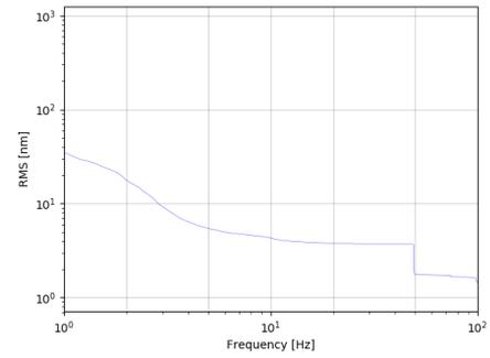
**Figure 2.18:** z RMS with seismometer not touching pipe in SQS-exp.
