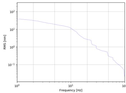
**Figure 2.31:** z RMS with seismometer below SQS-exp chamber.
