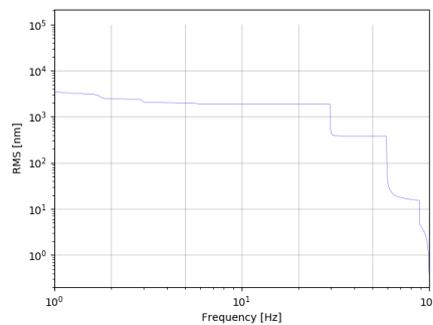
**Figure 2.8:** z RMS measured on top of the table with pumps in SCS-exp.
