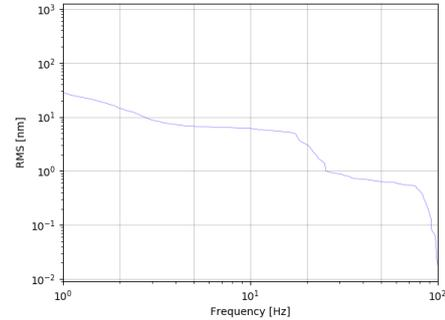
**Figure 2.28:** E-W RMS with seismometer on top of table support for the beam pipe inside HED-exp.
