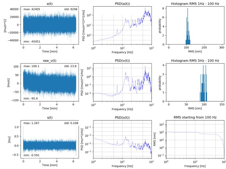
Figure 2.22: Data of the horizontal measurement of the vent pipe in SCS-exp.
