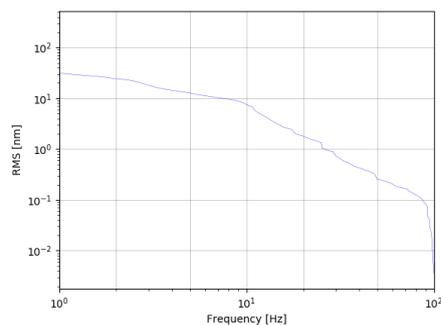
**Figure 2.25:** z RMS with seismometer below table support for the beam pipe inside HED-exp.
