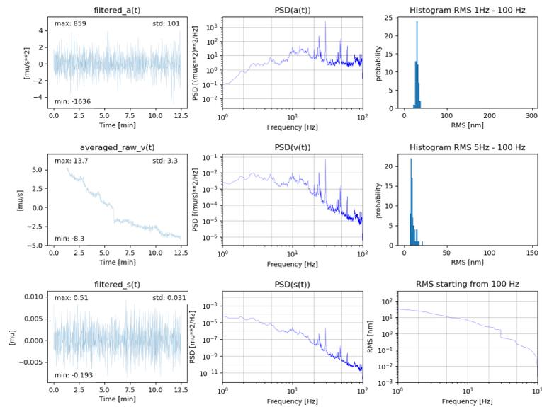
**Figure 2.5:** Measurement in the vertical direction inside the SCS-exp room.
