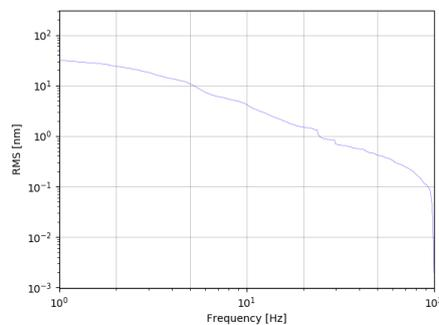
**Figure 2.15:** z RMS with seismometer touching pipe from SCS-exp.
