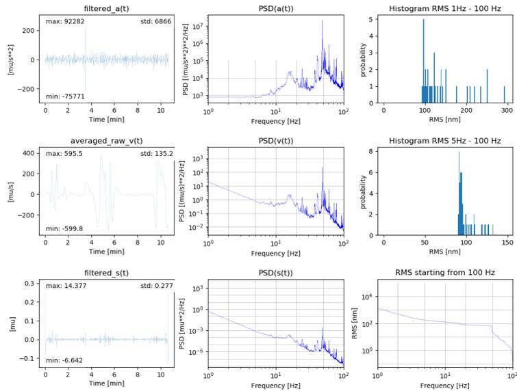
**Figure 2.4:** Measurement in the E-W direction inside FXE-rck in the corner nearest to the SPB-opt roof. Data is not very good, but still show a huge intensity around 49Hz.
