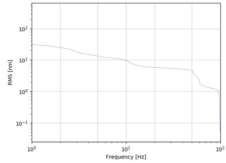
**Figure 2.30:** z RMS with seismometer on top of HED-exp chamber.
