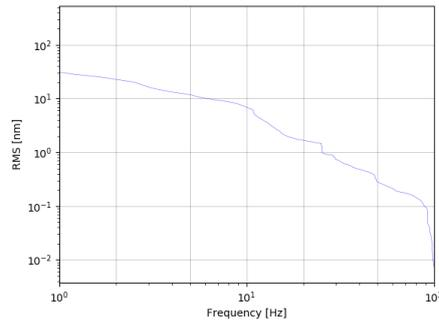
**Figure 2.29:** z RMS with seismometer below HED-exp chamber.
